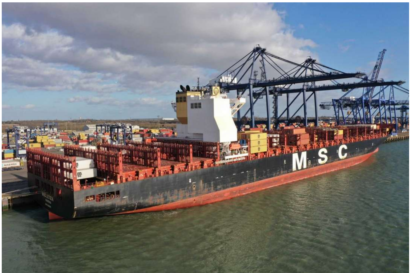
As can be clearly seen here, she has been fitted with an exhaust scrubber.
