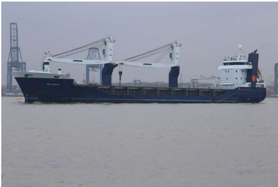
Passing Felixstowe inbound from Tananger, Norway to Parkeston number 3 berth on 22 nd February “Atlantic” is a fast general cargo ship capable of 18 knots and built to the Hartmann trader 18 design. Launched by Partner Shipyard, Police, Poland in January 2010, she was completed by Shipkits Groningen in November the following year. (Photo by David Hazell)
