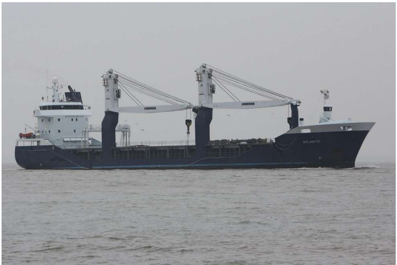
Passing Felixstowe inbound from Tananger, Norway to Parkeston number 3 berth on 22 nd February “Atlantic” is a fast general cargo ship capable of 18 knots and built to the Hartmann trader 18 design. Launched by Partner Shipyard, Police, Poland in January 2010, she was completed by Shipkits Groningen in November the following year. (Photo by David Hazell)
