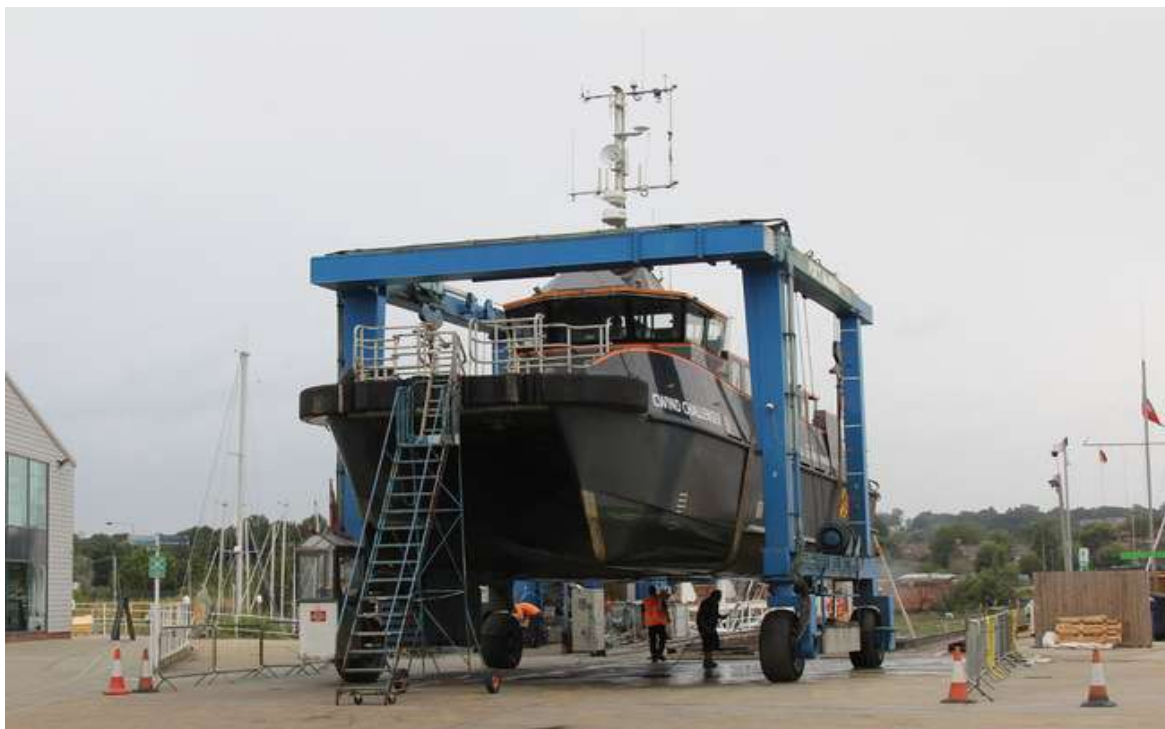
Now lifted out of the water for removal of marine growth etc. This composite resin built catamaran was constructed in Colchester by Ctruk in 2013, one of a number of successful vessels built by them. Several of which are for Cwind a subsidiary of Global Marine based in Chelmsford. (Both photos contributed)
