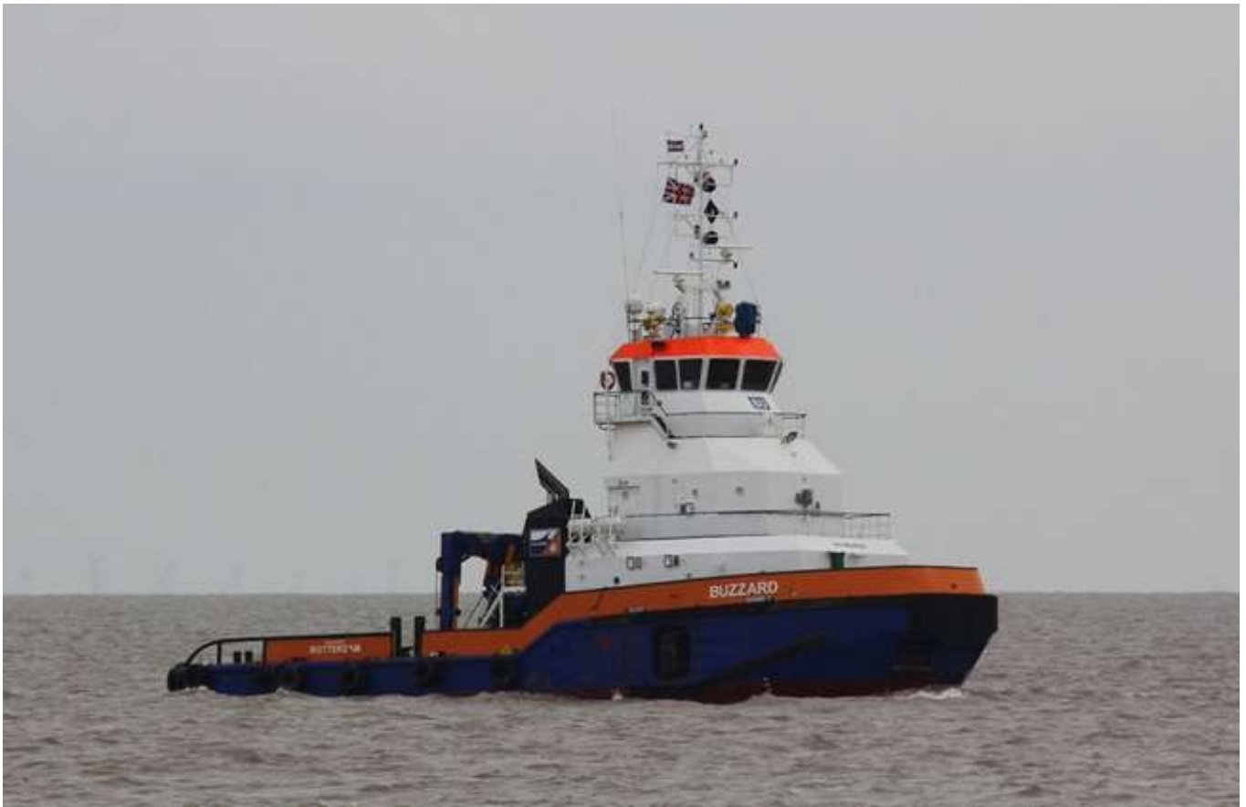
Van Oord's articulated pusher tug "Buzzard" working in the harbour on the dredging project on 28 th February. Her main task is "netting" boulders and discharging them for disposal onto "Goliath" for transfer to a hopper barge. She is also assisting with moving the dredger around. Launched in 2008 by Safe Shipyard, Gdynia she was completed by Damen, Hardinxveld the following year as "DMS Buzzard" for Damen Marine Services. Van Oord renamed her as above when they acquired her in 2010. (Photo contributed)
