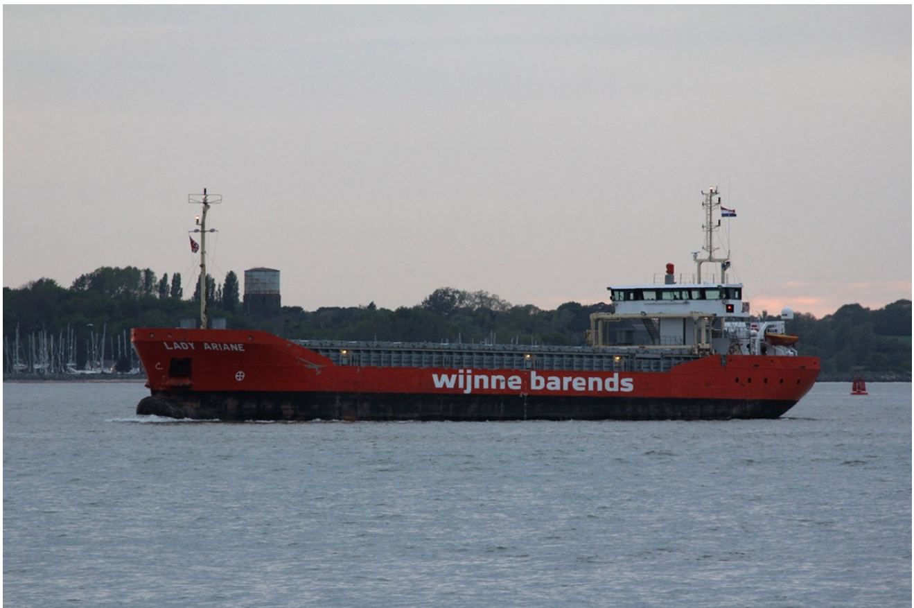
Having just left the River Orwell in the last of the day's light on 10 th May, "Lady Ariane" is heading for Ridham Dock, she had arrived in Ipswich from Riga on the 6 th . One of a series of twelve ships built by GS Shipyard BV, Waterhuizen which started operations on the former Van Diepen owned site in 2007. Completed to the design Sea River 3700 she was ready for service in November 2015. (Photo contributed)
