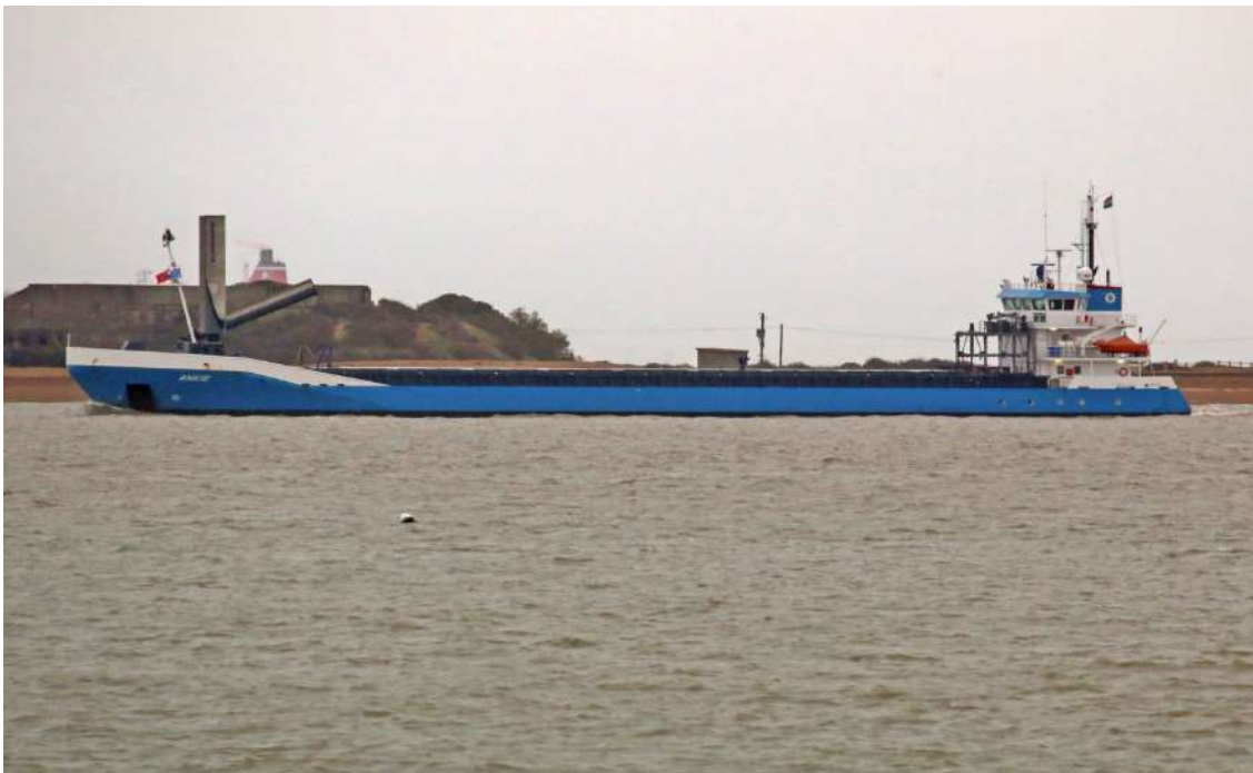
Passing Felixstowe inbound from Liepaja for Ipswich, Van Dam Shipping's “ Ankie ” lowers her retrofitted eConowind Ventfoil wind assisted system which was installed by Royal Niestern Sander in a January 2020 dry docking. Significant fuel savings have been realised by the 10 metre wings and the intention is to extend them by another six metres. The ship itself was launched into the Adriatic in November 2006 by Leda shipyard which is on the island of Korcula, Croatia. Completion was carried out by Peters, Kampen in January 2007. (Photo by Derek Sands)
