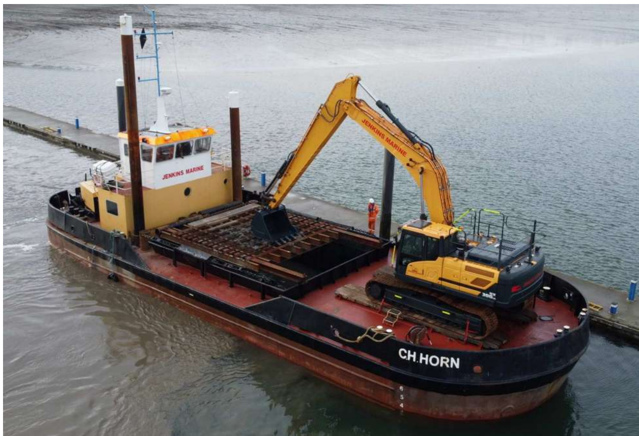
Recently upgraded by her owner Jenkins Marine's "CH Horn" getting into position to dredge at Woolverston Marina on 18 th January. Her fixed grab crane was removed during the upgrade and a modified tracked Hyundai excavator was installed. The excavator is equipped with a custom made lengthened dipper arm and has a 1.5m 3 bucket capacity, the excavator has an eco-friendly engine and weighs 30 tonnes. (Photo contributed)
