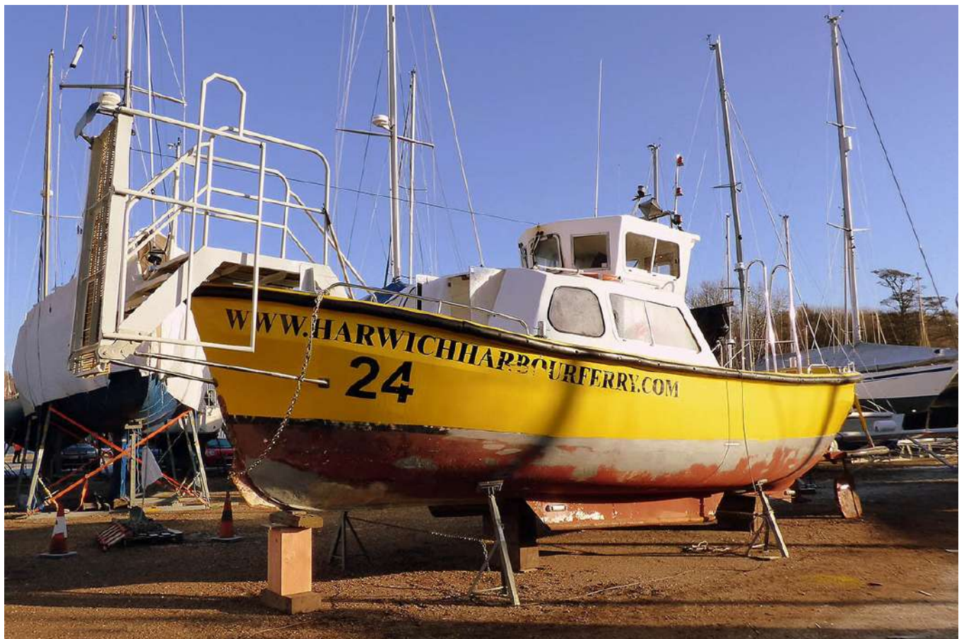
Harwich Harbor ferry undergoing maintenance at Levington Marina on 19 th January. Fibre glass renewal and painting of topsides and underwater. (Photo by Mick Warrick)
