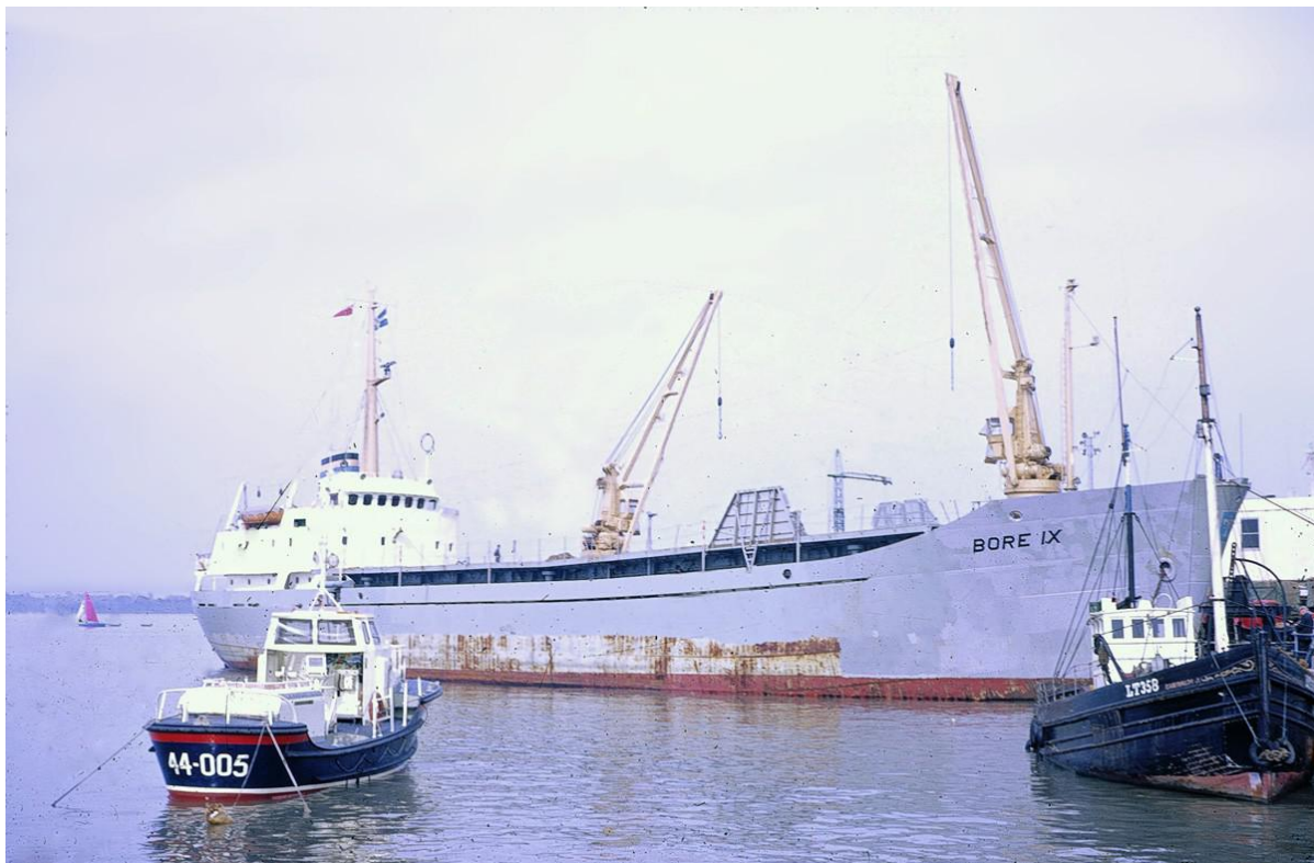
Somewhat of a rare photo of “ Bore IX ” at No.1 berth, Navyard Wharf, Harwich in 1968. Completed in July 1967 by Laivateollisuus, Turku for Bore Line she had a side door for pallet operations and was 1,297 gross tons. She had a short life as she capsized 14 nautical miles north east of Almagrundet lighthouse off the Stockholm archipelago on 19 th of January 1969 with six crew lost. She was on a voyage from Kemi in the north of Finland to London with cellulose. (Photo by Malcolm Cornes)
