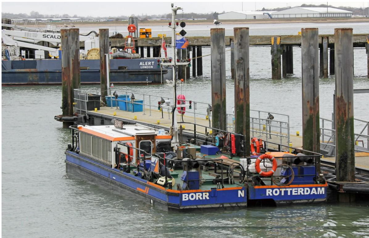
In a separate program, “ Borr ” seen at Harwich on 25 th March is undertaking water injection dredging in the River Stour. The work covers Harwich Navyard Wharf, Ha'penny pier, Trinity House berths, the windfarm pontoons at Harwich International (Parkeston Quay) plus Shotley and Mistley. She is able to be dismantled for road transport to various destinations and is owned by Van Oord. (Photos contributed)
