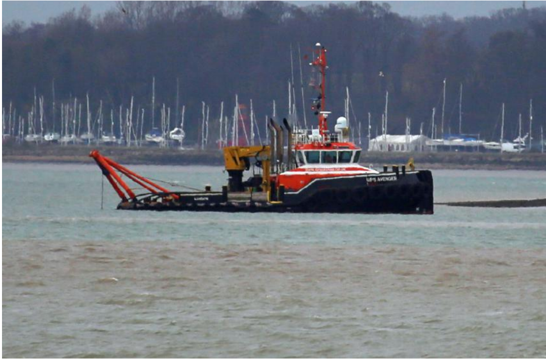
The tug carrying out ploughing and bed levelling off Berth 7 is “ GPS Avenger ” seen here on 28 th March. Built in 2013 she is a Damen Shoalbuster type, contracted by Damen, Hardixveld to Damen Kozle, Kedzierzyn-Kozle, Poland. The town is situated at the confluence of the Oder river and a tributary. The tug is owned by GPS Marine, London. (Photo by Derek Sands)
