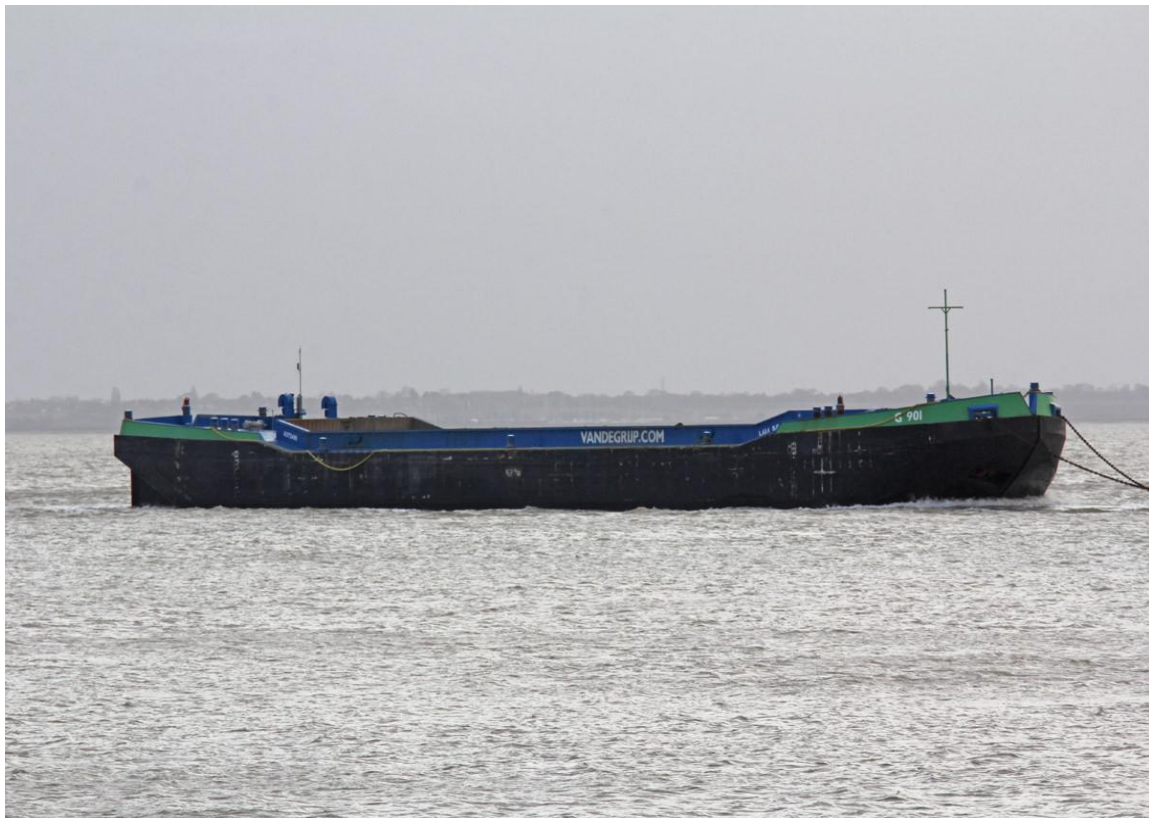
“G901” and her sister have radio controlled hopper doors and a length of 63.40m with a maximum draft of 3.55m and maximum load of 1,500 tonnes. No details of a builder could be sourced. (Photos contributed)
