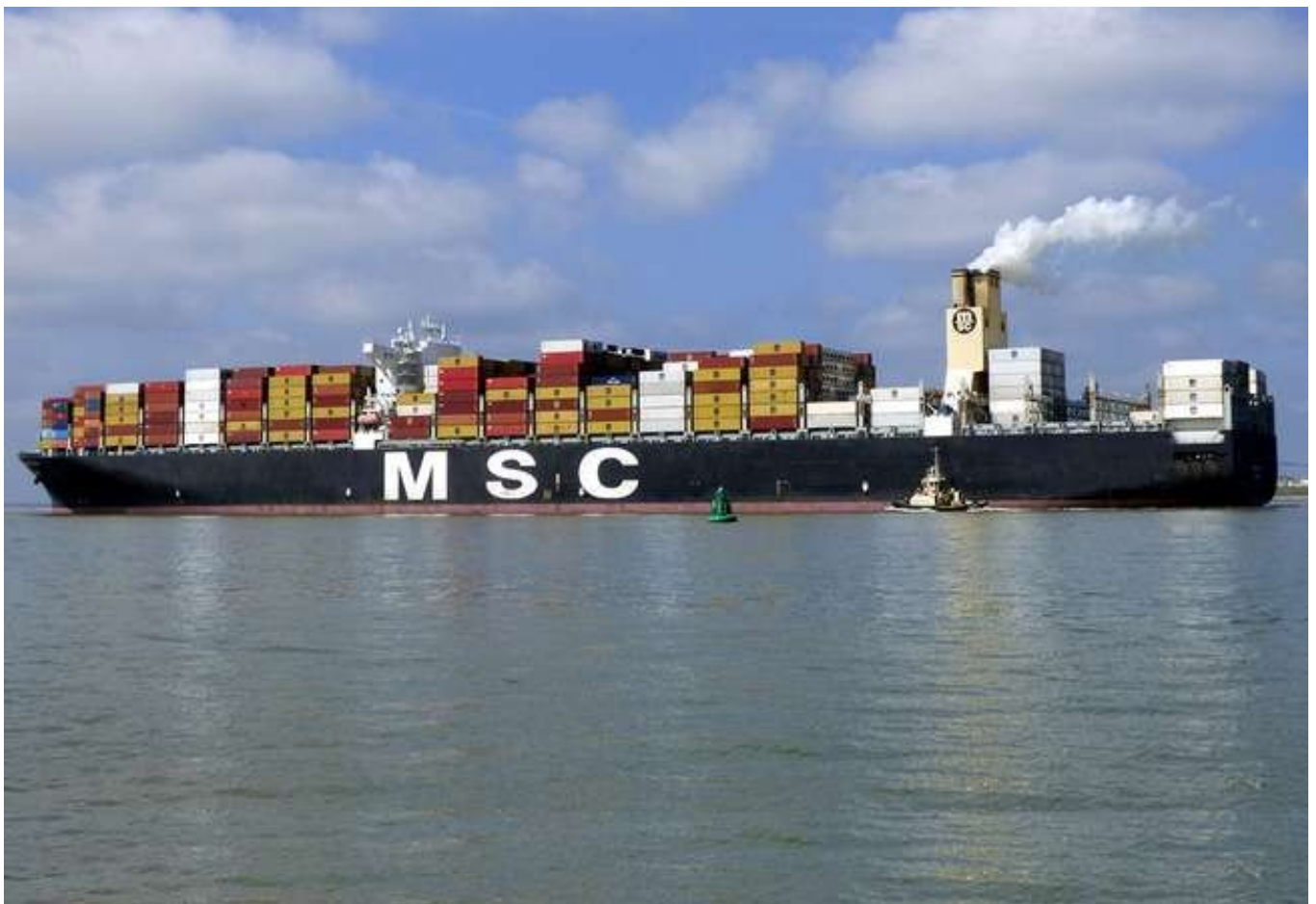
“MSC Gaia” sporting a modified funnel containing her retrofitted exhaust scrubber as she leaves Felixstowe on 7 th June. Her next port will be Hamburg as she does the rounds of European ports after arriving from Rotterdam two days earlier. The 366 metre vessel was completed in October 2010 by Samsung, Kojie, and has visited Felixstowe several times. (Photos by Mick Warrick)
