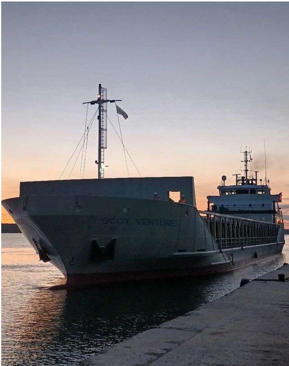
“Scot Venture” arriving from Inverness on 5 th July, she would sail for Rotterdam the next day. The normal cargo from Inverness is wood pellets. Built to the Tille Trader 3300 design by Tille SY at Kootstertille in 2002. (Photo by Steve Cone)
