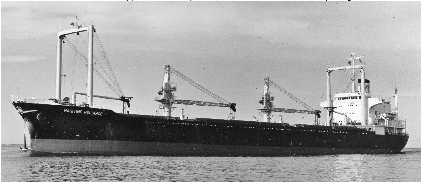
ABOVE: MARITIME RELIANCE is fitted with two swinging derricks and 2 deck cranes, as seen on arrival, 13/08/1972.
