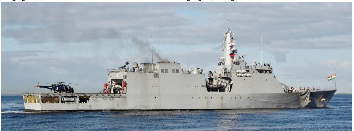
ABOVE & BELOW: Two views of INS SUMEDHA departing Fremantle in tranquil conditions 18/08/2022. The tarpaulin hanging over the starboard side shoulder was for the attending tug to push against and therefore not mark the hull.
