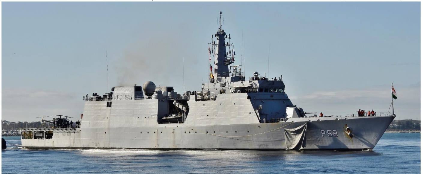
ABOVE & BELOW: Two views of INS SUMEDHA departing Fremantle in tranquil conditions 18/08/2022. The tarpaulin hanging over the starboard side shoulder was for the attending tug to push against and therefore not mark the hull.
