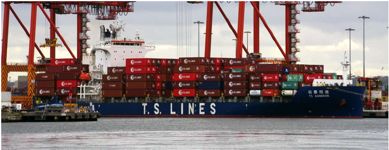
TS Bangkok , IMO 9784233, 17,449 GT, 172m loa, 21,361 dwt, 1,808 teu, flagged in the Marshall Islands and built in 2017 at China Shipbuilding Corporation in Keelung and one of many sisters in the TS Lines fleet. She was alongside at ESD over the 17 – 18/3 and now operates with the on TS Lines CA3 service from the Chinese ports of Qingdao, Shanghai, Nansha and Shekou with sisters TS Nansha , TS Qingdao , TS Hochiminh and TS Pusan with this service using Patreck's at East Swanson Dock. Her registered owner is TS Empire Holding Ltd of Taiwan, beneficial owners, managers and commercial operators are TS Lines Co Ltd of Taiwan with Fleet Management of HK her technical manager. Photo from Dale Crisp
