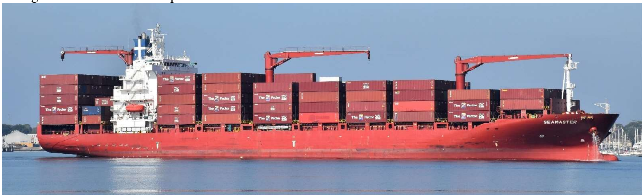
Seamaster , IMO 9625920, 20,239 GT, 170m loa, 24,129 dwt, 1,756 teu – 3 x 40mt cranes, flagged in Malta and built in 2013 at SPP Shipbuilding at Sacheon, South Korea. Having joined the Zim / Gold Star Line's new C3A service ( same as the H Cygnus ) from Chinese ports, she was alongside at ESD over the 21 – 22/3. Her registered owner is the wonderfully named Pansy Shipping Ltd of Greece with Eastern Mediterranean Shipping of Greece her beneficial owner and manager and she has gone on charter to ZIM / GSL for an unknown period. Photo from Paul Finnigan.
