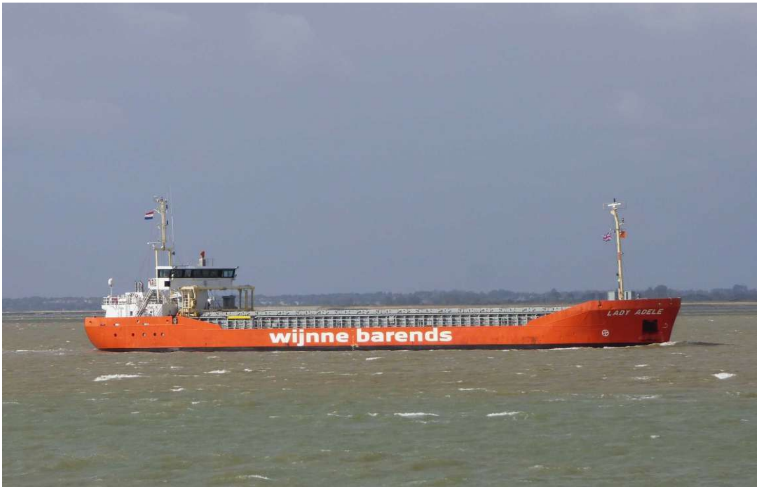
Wijnne Barends was founded in 1855 in Groningen and since 2003 is part of the Spliethoff Group. They had a series of twelve ships of this type built by the GS Yard at Waterhuizen. “Lady Adele” was the fifth one launched of the series and was completed in May 2015. She conforms to the Sea River 3700 design with a deadweight of 3,700 and she is eighty eight metres overall with a beam of nearly thirteen and a half metres. She has an eight cylinder main engine with a fixed propeller and is capable of ten knots. She is seen here inbound for Ipswich on 11 th September. She sailed the following day for orders and stayed at the Cork anchorage for 5 days until leaving for Amsterdam. (Photo by Mick Warrick)
