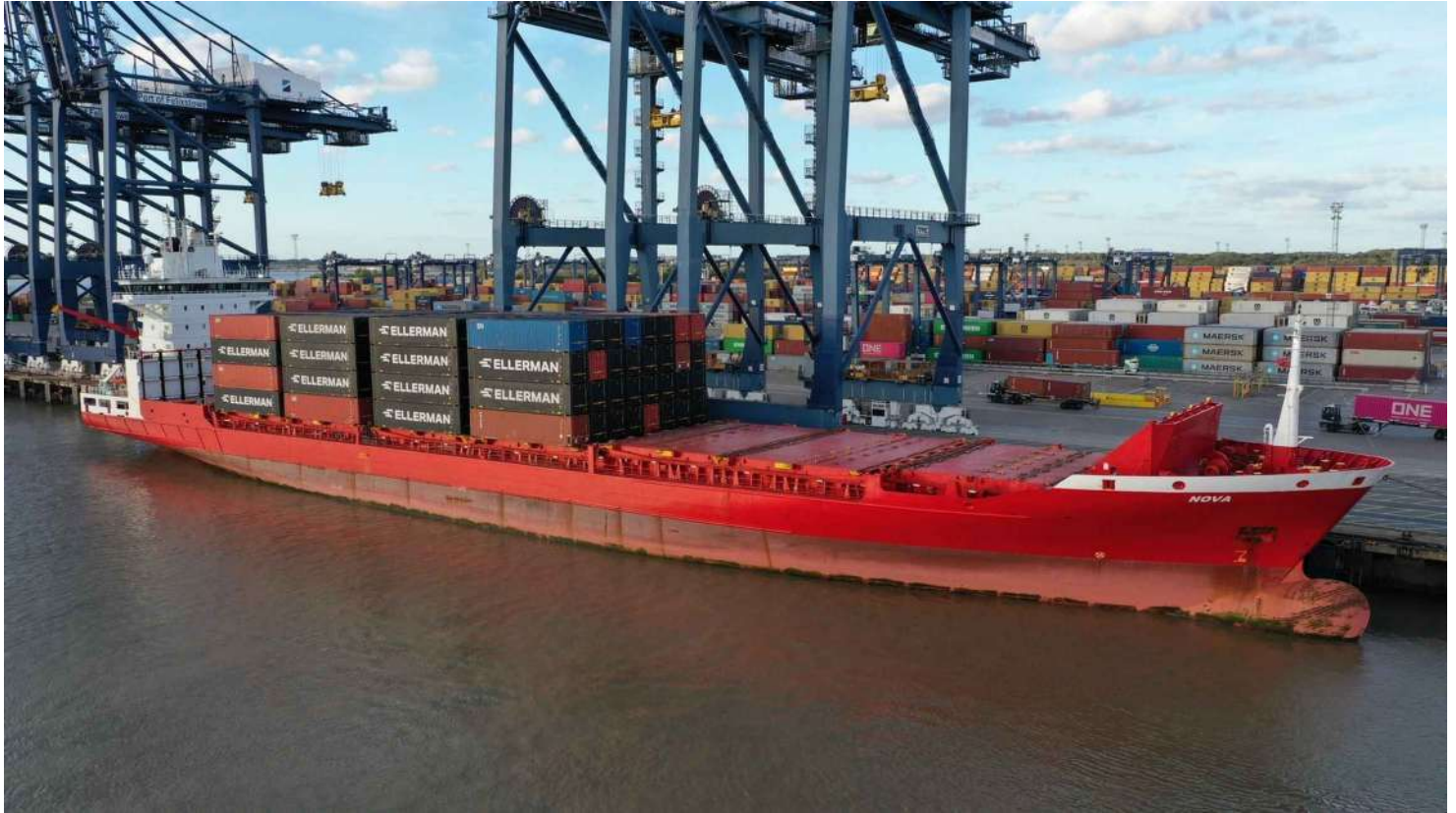
“ Nova ” waiting to start loading at Trinity Terminal on 25 th September. She had arrived from Tilbury where she had loaded the Ellerman containers. Built by J.J. Sietas, Neuenfelde, Hamburg in 2002 as “ Containerships VII ” for Finnish owners. Retrofitted with an exhaust scrubber in 2011 she went to German flagged operators in 2022 as “ Nova ”. (Photos contributed)
