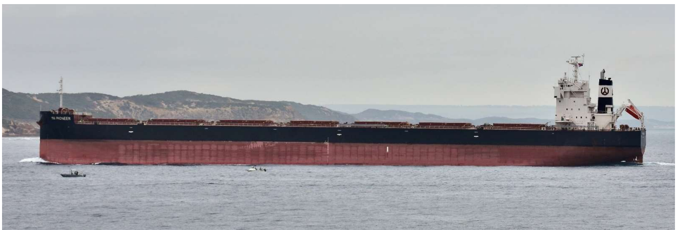
YM Pioneer , IMO 9902548, 43,424 GT, 81,898 dwt, 229m loa, Kamsarmax flagged in Liberia and built in 20121 approaches Port Phillip Heads bound for Bulk Grain Pier 3 where she loaded 60,000mt of barley for the UAE port of Jebel Ali over the 27/1 – 1/2. Photo from Graham Flett.
