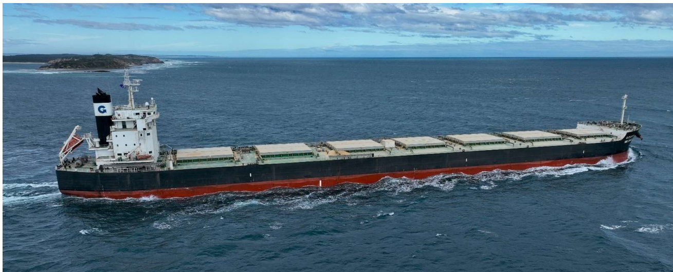
BBG Grace , IMO 9702704, 43,007 GT, 229m loa, 81,952 dwt, Kamsarmax flagged in HK and built in 2015 at Tsuneishi H.I. at Fukuyama. After ballasting from HK and a few days awaiting a berth, she loaded 55,000mt of wheat at Bulk Grain Pier over the 11–15/3 for the Vietnamese port of CaiMep a/c shipper Viterra. Her registered owner is CL Heifei Ltd of HK, beneficial owners are the China Development Bank of China, of Greece, managers are An Shun Ship Management of HK and her head charterer and operator is BG Shipping Co – Beibu Gulf Shipping, a HK based company controlled by Guangxi Province owned Beibu Gulf Port Group. Photos from Kevin Finnigan / Owen Foley.
