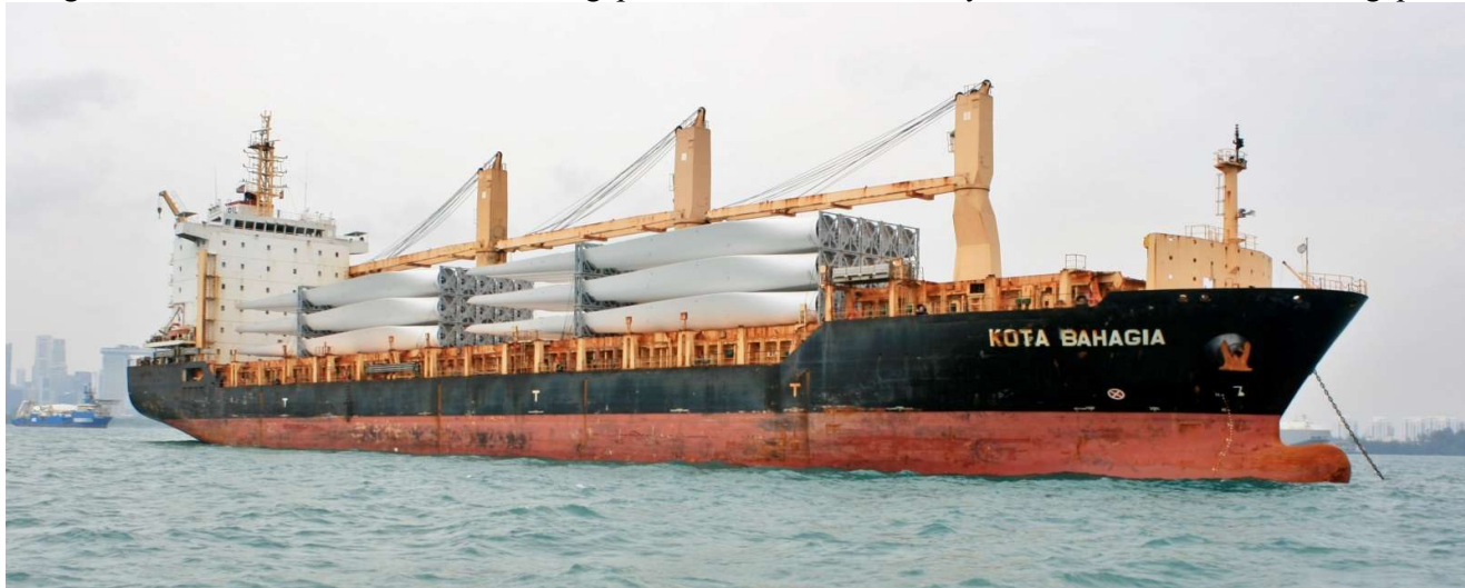
Kota Bahagia , IMO 9593672, 18,169 GT, 161m loa, 24,964 dwt, general cargo vessel – 1,497 teu 1 x 60 / 2 x 100mt cranes, Singapore flagged and built in 2011 at Dalian Shipbuilding as one of seven sisters. This vessel was over two months late after she sustained a fire in hatch 1 whilst in the port of Napier and was eventually alongside at 1 South Corio over the 26 – 27/2 discharging some wind blade compnenets loaded in China. She is registered to PSI 2 Pte Ltd of Singapore with her beneficial owners, managers and commercial operators being Pacific International Lines of Singapore. Photo from Harvey Wilson and taken in Singapore.
