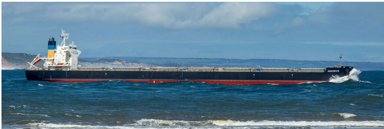
Amadeus , IMO 9749855, 44,425 GT, 229m loa, 81,676 dwt, Kamsarmax flagged in Panama and built in 2016 at the Namura Shipyard in Imari, Japan. She was alongside at BGP3 over the 31/10 – 4/11 loading 59,000mt of wheat for the Malaysian port of Port Kelang a/c shipper Cargill. Her registered owner is Blue Castle Investments Inc of Panama, beneficial ownership and management is from Goulandris Brothers Hellas Ltd of the UK with tech management from Anglo Eastern Ship management of Hong Kong. Photo from Lester Hunt.
