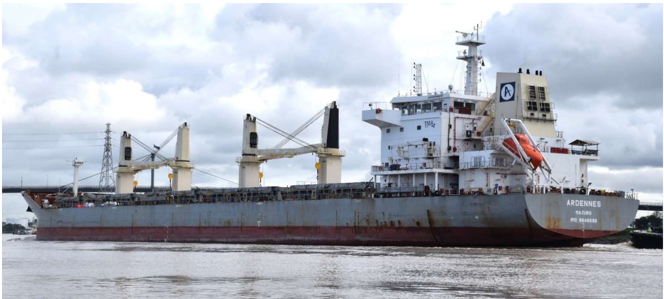
Ardennes , IMO 9646699, 24,247 GT, 180m loa, 36,062 dwt, Seahorse35 class bulk carrier flagged in the Marshall Islands and built in 2013 at Nanjing's Jinling Shipyard. On voyage charter to SwireBulk, she was alongside at Appleton Dock discharging steel products from Kaohsiung, Taiwan having part discharged in Brisbane prior. She is registered to Stallion One Shipping Co SA of the Marshall Islands, beneficial owner
