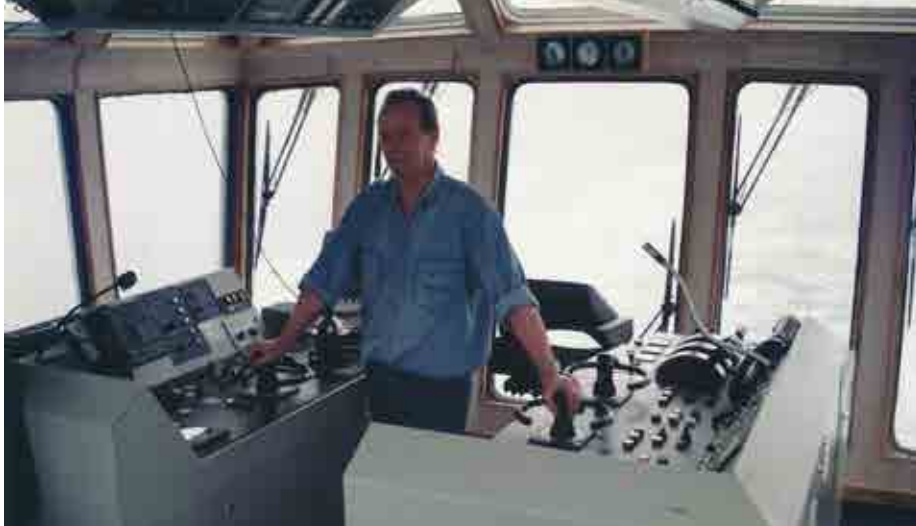
Captain Aalbers steering RT PIONEER with the two forward controls. The aft control is in the centre position photo: Hans Hoffmann
