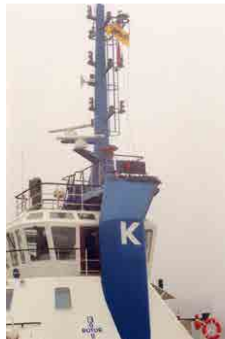
Wheelhouse with navigation mast photo: Job van Eijk
