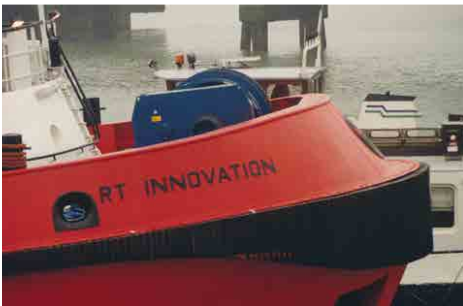
Bow fendering and forward winch
