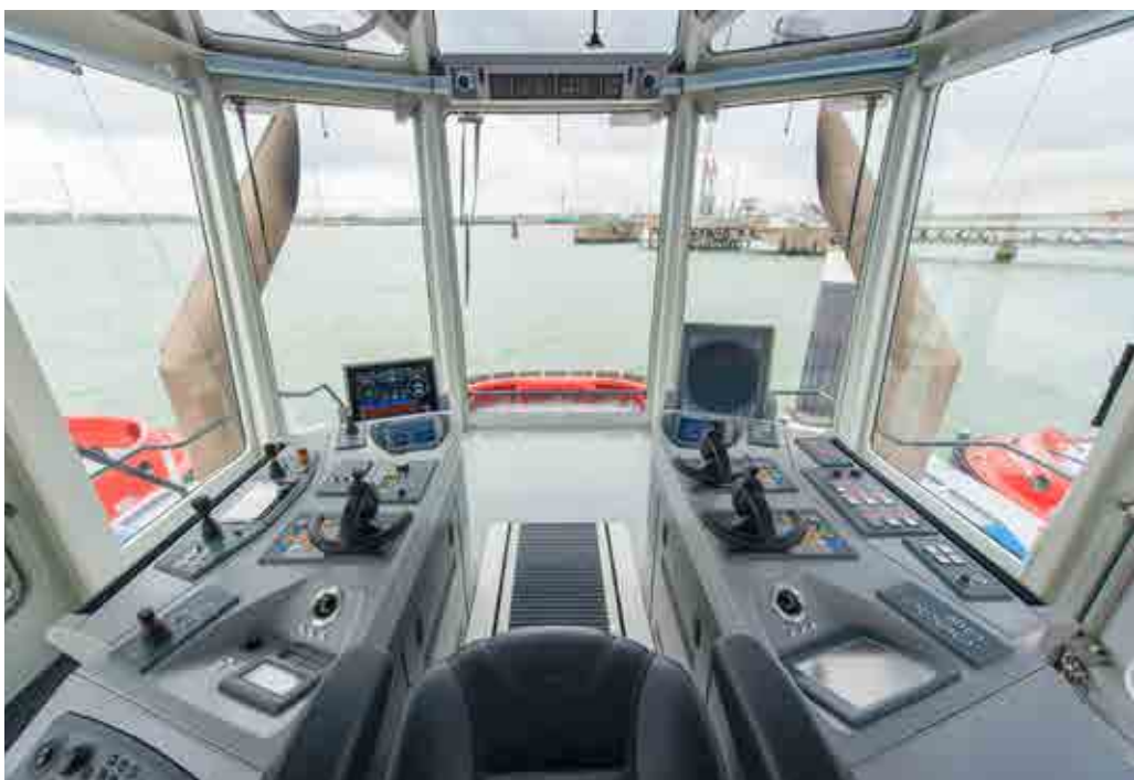
The Alphabridge Tugboat Console on RT EVOLUTION - also note the almost unobstructed all-round view
