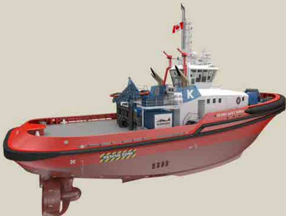
Artist's impression of the dual fuel methanol-diesel stern drive for Canada artwork: courtesy Robert Allan Ltd
