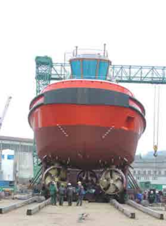
Visible are the sponsons, lack of docking struts, the position of the 3 schottel thrusters photo: Kotug
