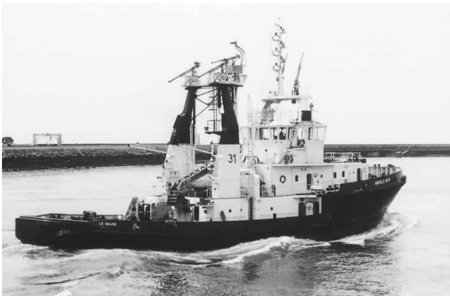
ABEILLE 31 and sister 32 were designed and built especially for the oil terminal at Antifer, north of Le Havre. These tugs were fully equipped for fire-fighting including a real fire ladder
