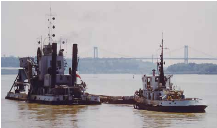
DRAGUE No. 7 - a bucket dredger at work in the Gironde River. The dump barges are handled by R-6 and R-8
