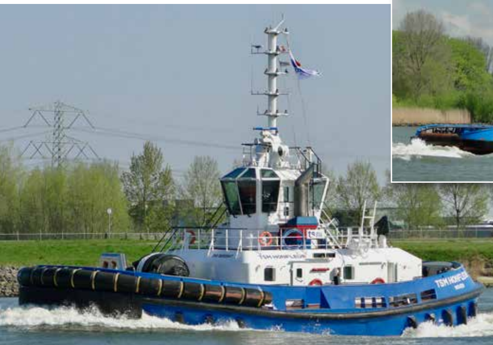
TSM HONFLEUR was delivered to Thomas Services Maritime of Rouen. The 80 ttp - 2021-built Damen RSD TUG 2513 design - seen here in The Netherlands during trials - works mainly at the river terminals in the River Seine west of Rouen
