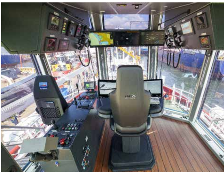
Wheelhouse BOSS with IBS controls and rotating helmsman's chair
