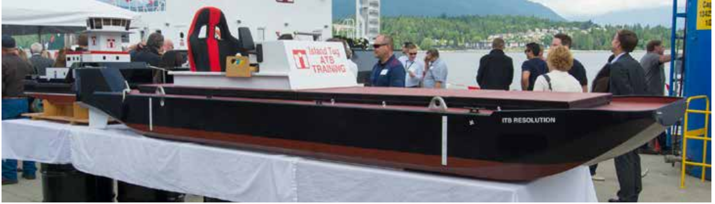
Burchett's scale model of the tug and barge combination ISLAND RAIDER and barge ITB RESOLUTION was commissioned by Island Tug & Barge for training of the crew as the propulsion system as well as the connecting system – a 'pin' boat - was new to Island T&B. The operator sits in the seat on the barge with a full set of controls for azimuthing drives and the barge's bow thruster photo: Alan Haig-Brown
