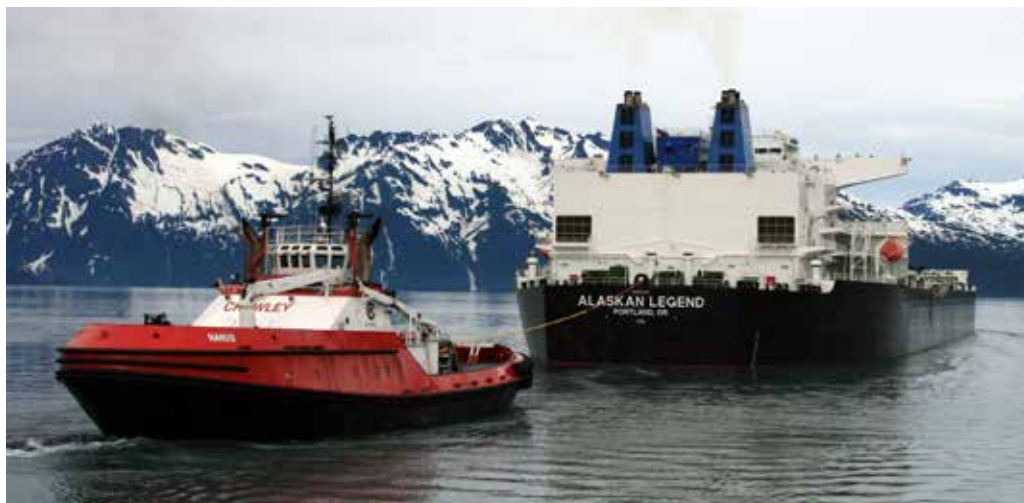
The Crowley Voith Tractor NANUQ as tethered escort of the tanker ALASKAN LEGEND at Valdez
