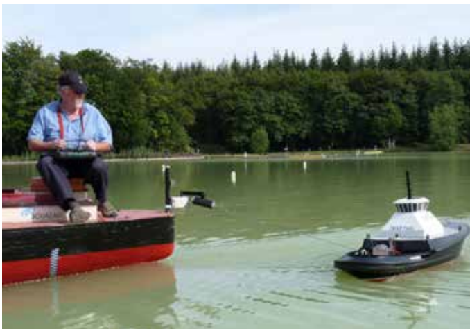
Testing escort manoeuvres using a remote-controlled model of a Voith Tractor connected to a free running manned tanker model
