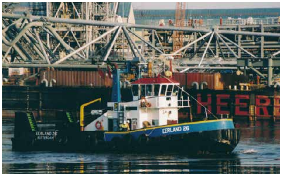
EERLAND 26 assisting ASIAN HERCULES II. In the background part of the flare boom to be lifted. EERLAND 26 is the former JANUS, the first-ever Schottel tractor tug (see TugeZine 11 for a full report on this tug and Schottel)
