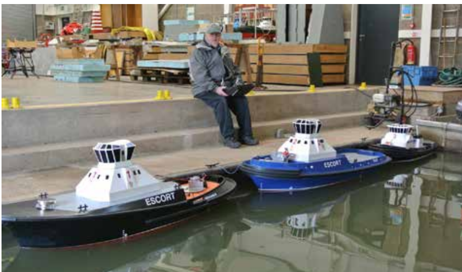
Three models used in the testing of the Auto Position Escort Winch - l to r Voith and ASD with the Auto winch, ASD with conventional bow winch
