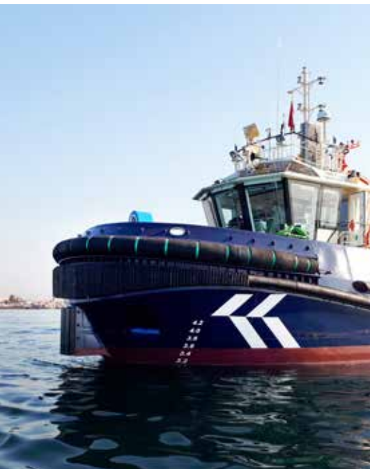
Note bow pushing pad below bow fendering typical for the YENICAY design
