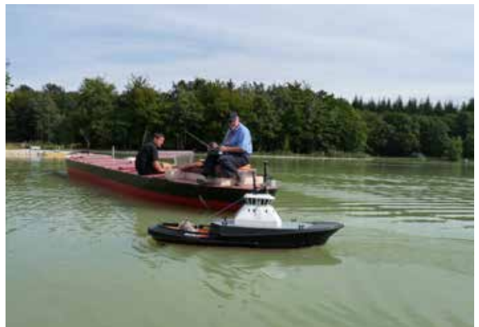
Testing escort manoeuvres using a remote-controlled model of a Voith Tractor connected to a free running manned tanker model
