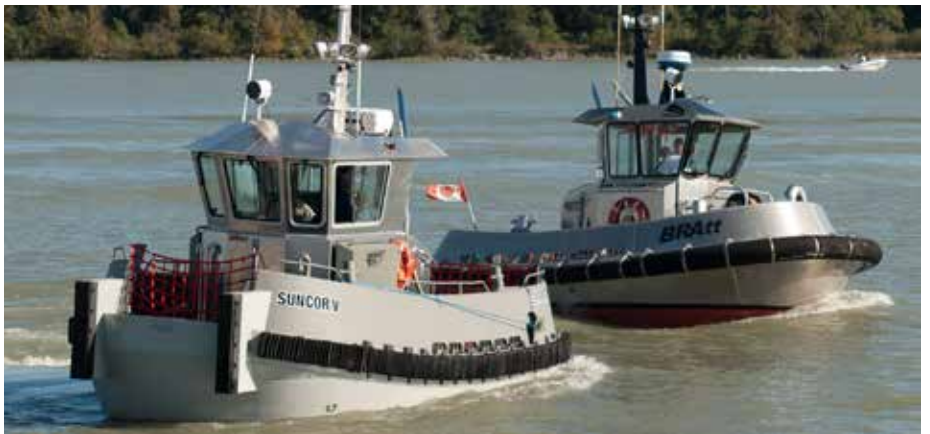
SUNCOR V with BRAtt behind. SUNCOR V differs in that it is not a training tug hence the tug is fitted with pushing pads and is steel-hulled
