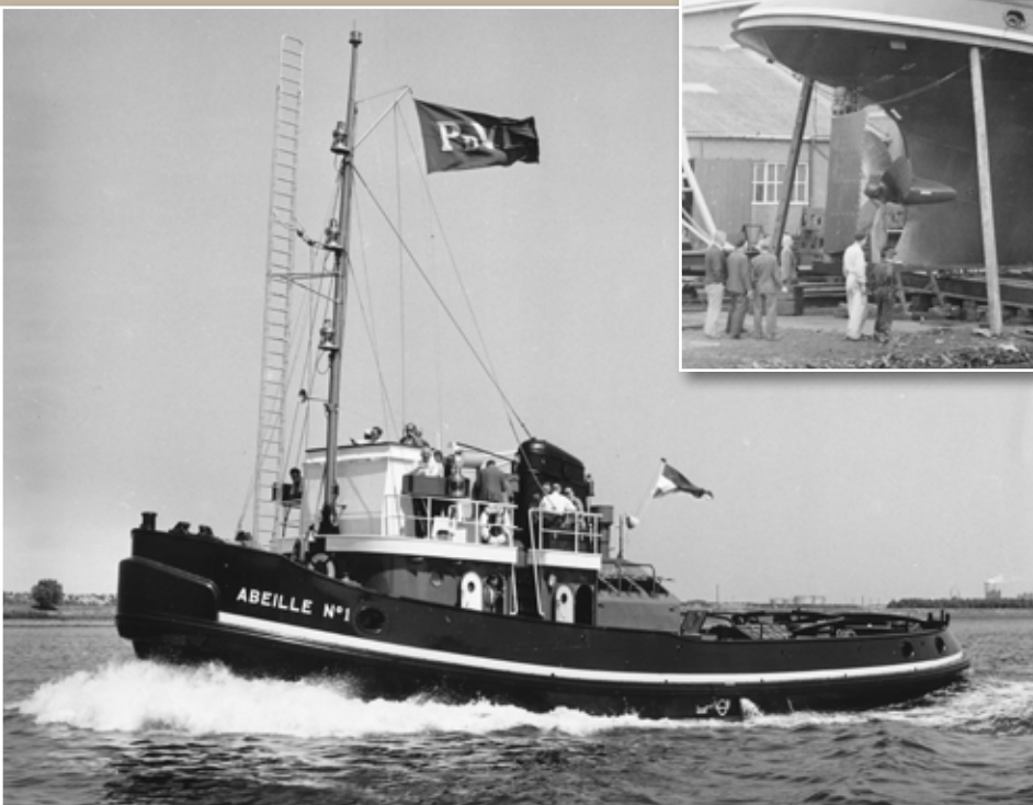
ABEILLE No 1 during the hand-over trials. The 500 bhp tug was delivered to the owners in July, 1959, by Shipyard De Vries Lentsch, at Alphen a/d Rijn. The tug and its sisters ABEILLE No 2 and ABEILLE No 3 (this was the first to be delivered actually) were classed for English Channel and French coasting service. In later years the steering stand was replaced by an enclosed wheelhouse. ABEILLE No 1 was spotted at Perama on 20 April, 2022, named CHIOS I
