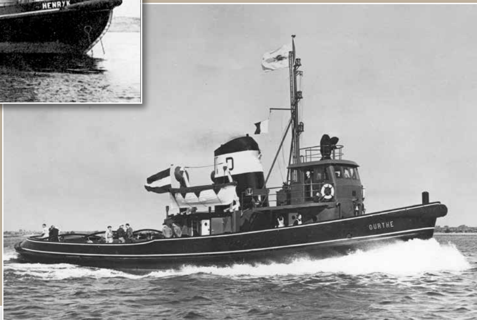
OURTHE and sister LEIE were built in 1953 by IHC Holland for account of the Société Générale de Dragage, Belgium. The steam tugs measured 26,50 x 7,30 x 3,55 m. Engine output 400 ihp photo: IHC Holland
