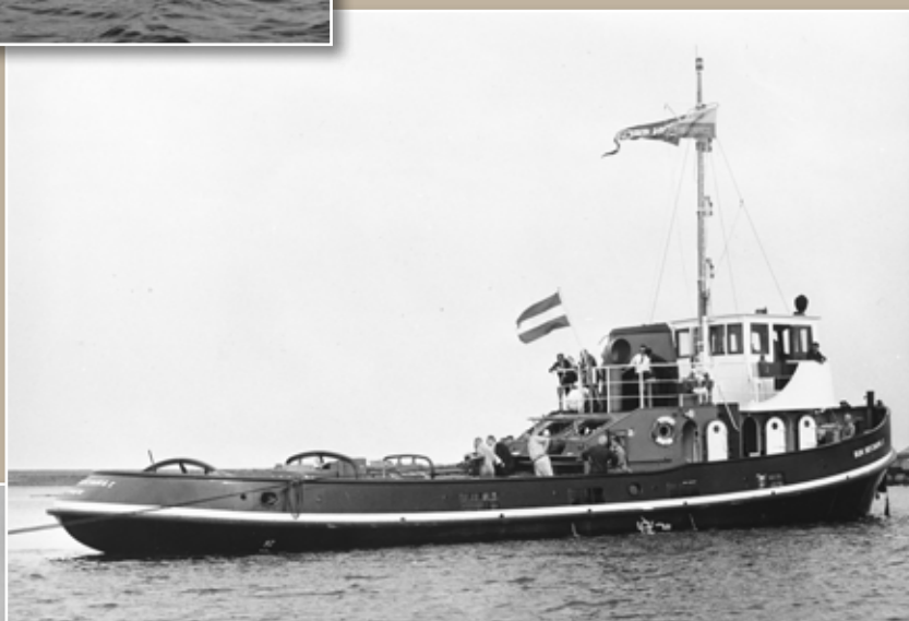
Another French tugowner ordering from The Netherlands was Cie. Louis Thomas. BON SECOURS 1 is seen preparing bollard pull tests. The 500 bhp tug was built by Bodewes Martenshoek and delivered in June, 1964
