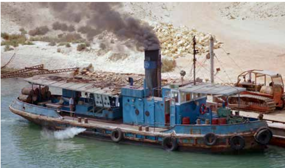
The 350 ihp DARFIL 153 - seen here on 13 September, 1988 - is one of a series of identical tugs built by IHC yards for account of the Compagnie Universelle de Canal de Suez. Sister DARFIL 138 was subcontracted to the Biesbosch yard and delivered in 1951. Dimensions were 22,99 x 6,05 x 2,79 m. photo: Hans Hoffmann
