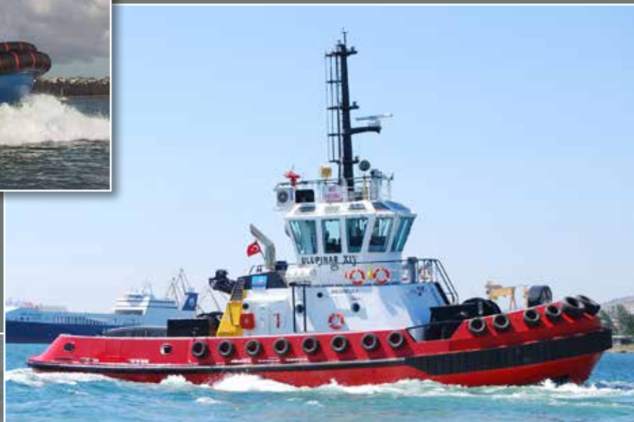
ULUPINAR XIV is a RAport 2400-Mk2. Since 2008, 20 Ulupinars have been built by Sanmar. Presently sailing as STATESMAN for SMS Towage. 24,4 x 9, 2 m, 3.346 bhp, 50 ttp
