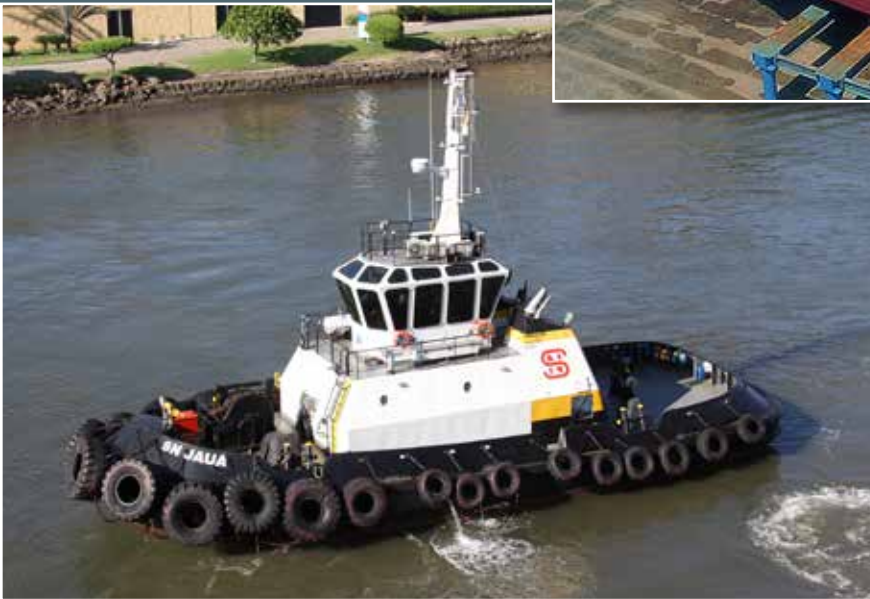
The RAport 2400-Mk1 SN JAUJA seen at Vitoria, Brasil, in 2019. Built 2004 by Detroit Brasil for account of the Grupo H. Dantas, the tug flies the flag of Dantas subsidiary Sulnorte. 24,4 x 9,2 m, 2.828 bhp, 40 ttp. Sistership is SN CAETE
