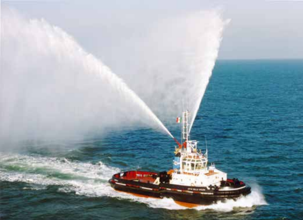
The second-ever Damen ASD tug was the first to be built in The Netherlands. In 1993 the design was presented to the tug industry in Rotterdam. Seen here running trials photo: Damen Shipyards
