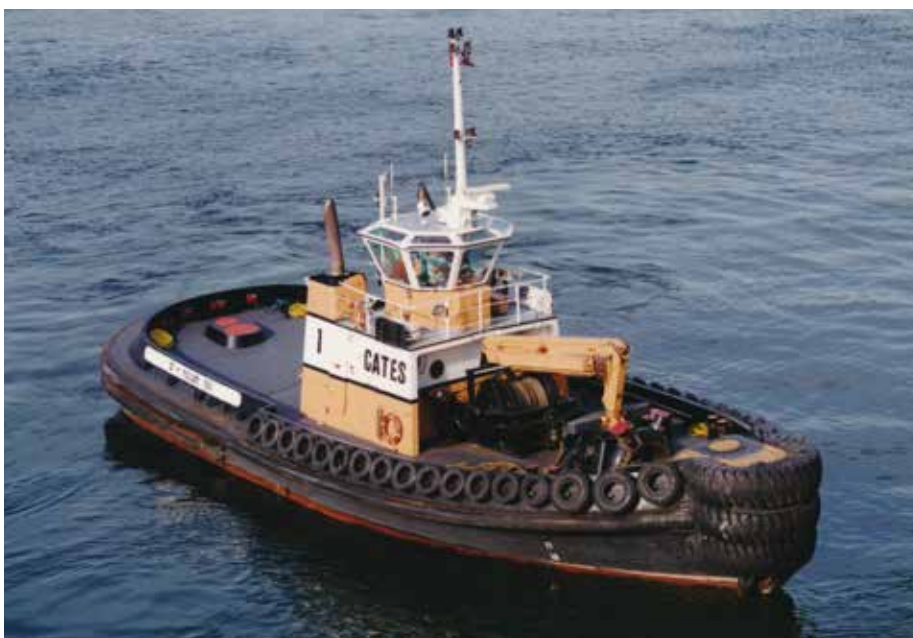
CHARLES H. CATES I at Vancouver 12 May 1994 with het line-handling / hawser crane in the stored position photo: Hans Hoffmann
