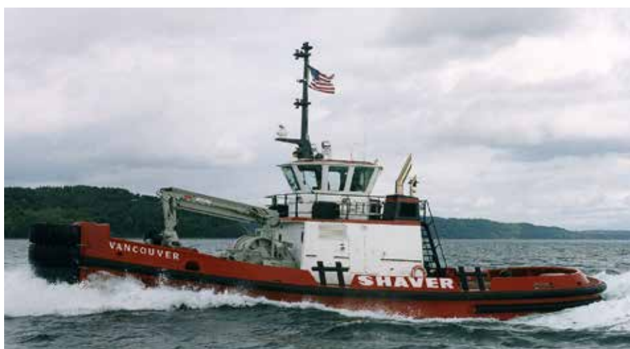
VANCOUVER was delivered to Shaver Transportation in 1993. Dimensions are 22,9 x 8,5 m. Currently typified as a Cate 23 / 35 design
