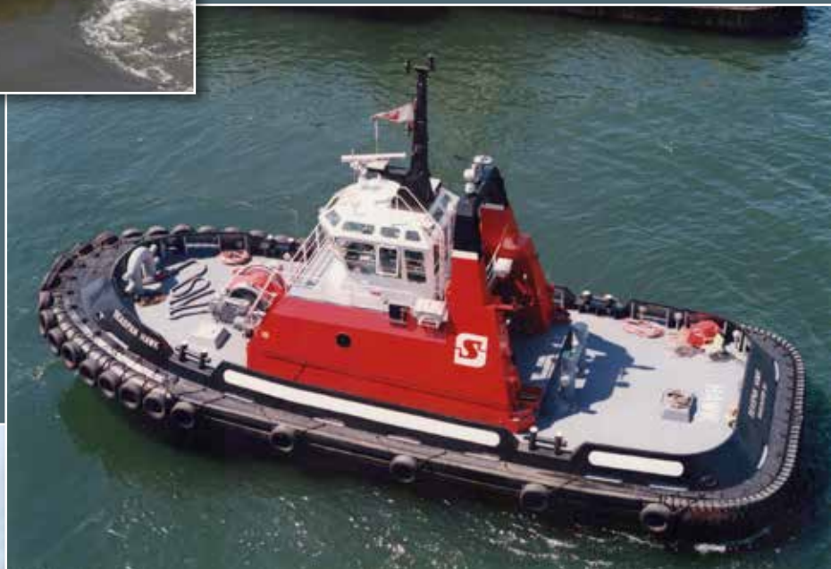
SEASPAN HAWK is a RAport 2400-Mk1 seen here working at Vancouver on 7 July, 1994. Built in 1993, 23,3 x 9,8 m, 3.100 bhp. Sister is SEASPAN FALCON
