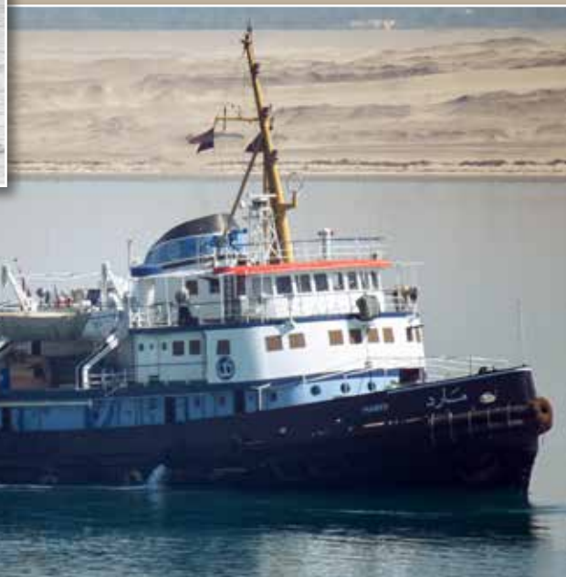
MARED (pictured) and sister SHAHM were completed by IHC in 1960. The diesel-electric 6.400 hp tugs were built for account of the Suez Canal Authority. Dimensions 42 x 12 x 3,30 m. Speed 10,5 knots photo: P. Kerkvliet
