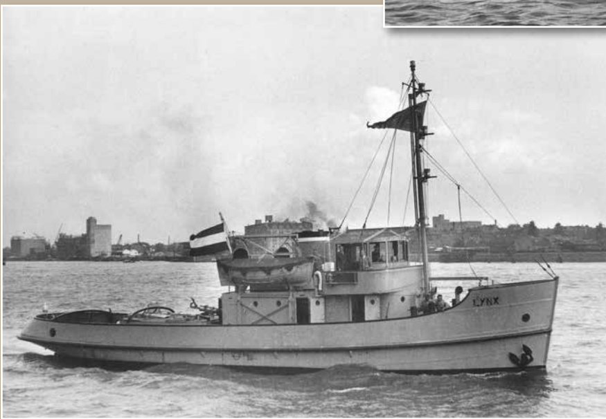
LYNX and sister PHÉNIX were built by IHC in 1948 for account of S.A. Ossude, Paris. The seagoing motor tugs had an output of 350 hp. Dimensions 24,25 x 6 x 3,30 m photo: coll. Job van Eijk
