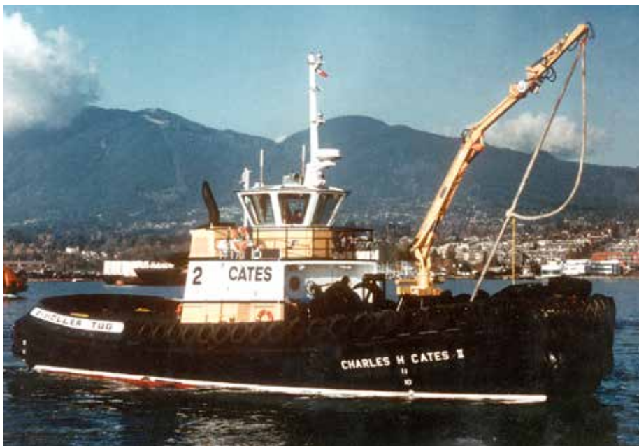
CHARLES H. CATES II - the first stern drive tug in Canada - demonstrating the use of the hawser crane photo: coll. Robert Allan Ltd
