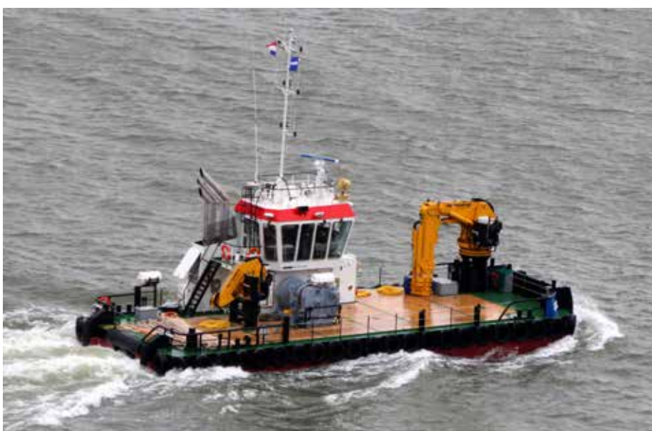
LAMINE CAMARA delivered in 2022 is an example of a Damen Multicat 2409. The vessel is required to fulfil multiple functions in the port of Kamsar. These include maintenance of the nav buoys but also shiphandling. The combined towing / anchorhandling winch allows for work over the bow or over the stern
