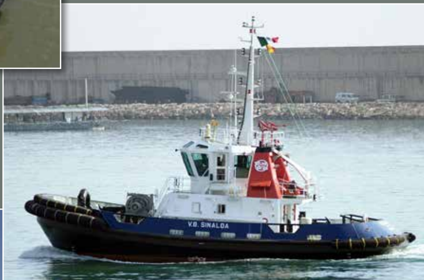
VB SINALOA is one of a series of 11 RAport 2400-Mk2 tugs built for Boluda subsidiary Compania Maritima del Pacifico, Mexico by Union Naval Valencia in Spain. UNV designated the class as UNV 352-SD. 23,80 (oa) x 11,00 (mld), 4.259 bhp (3.132 kW), 53 ttp ahead / 48 ttp running astern
