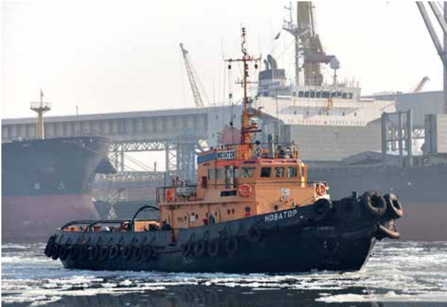
NOVATOR was built in 1982 by Brodogradiliste Tito. 35,83 / 32,07 x 9,30 x 4,50 m. Draught 3,04 m. 2x 6 cyl. Sulzer 6-ASL-25/30 total output 2.520 bhp. 1982-92 Russian Government. 1992 to Odessa Commercial Sea Port
