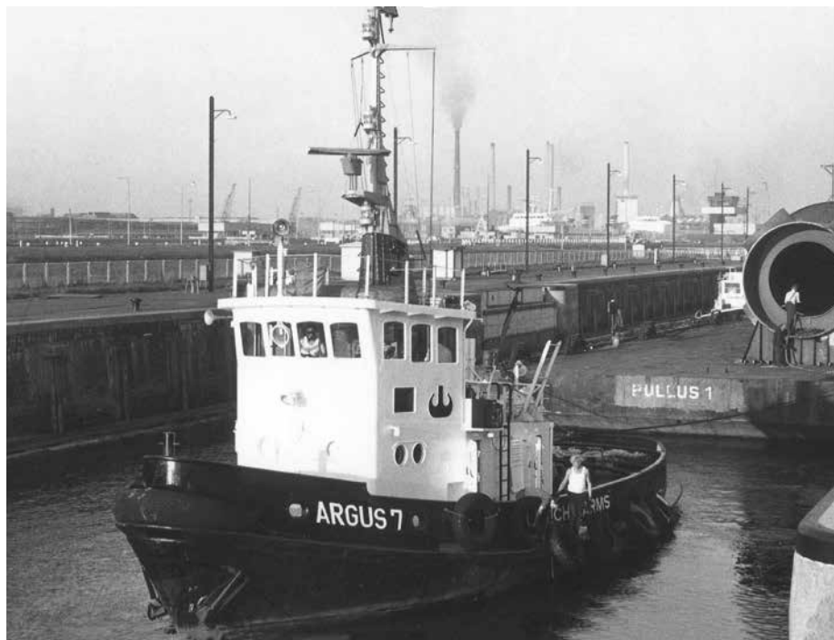
ARGUS 7 is one of a series built for sheerlegs assistance in port as well as for sea transport - seen here towing the Harms pontoon PULLUS 1 photo: Ger de Vries
