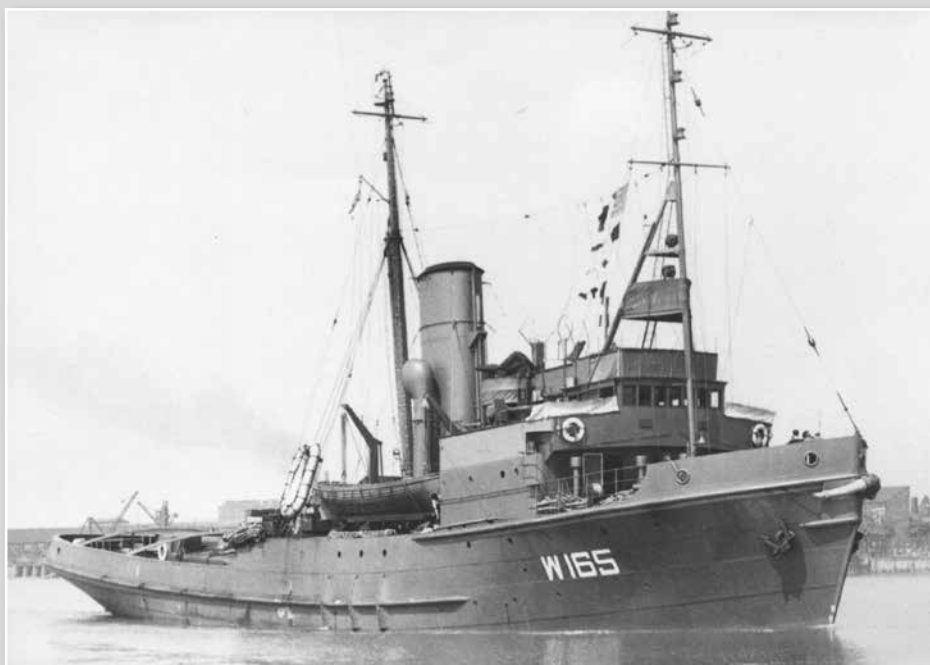
ENVOY, lead ship of this class of rescue tugs was built in 1944 by Cochrane, Selby. 868 t. displacement, 1.700 ihp triple expansion. 13 knots. Armed with 1x 3" AA, 2x 20 mm AA and 2x 2 machine guns
