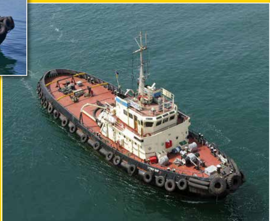
STIVIDOR was built by BrodogradilisteTito for the Russian Government. 35,44 / 30,00 x 9,30 x 4,50 m. Draught 3,15 m. 2x 7 cyl. B&W Alpha 7-26MTBF-40, total output 2.300 bhp. 1992 to Odessa Commercial Sea Port
