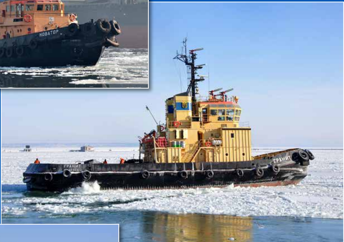
GRANIT dates from 1982, built by Hollming Oy, Rauma. 39,90 / 38,20 x 12,50 x 7,00 m. Draught 4,90 m. 2x 6 cyl. Wärtsila 6R-32, total output 4.970 bhp. Twin Kort nozzle-rudders. 1982-92 Russian Government. 1992 to Odessa Commercial Sea Port
