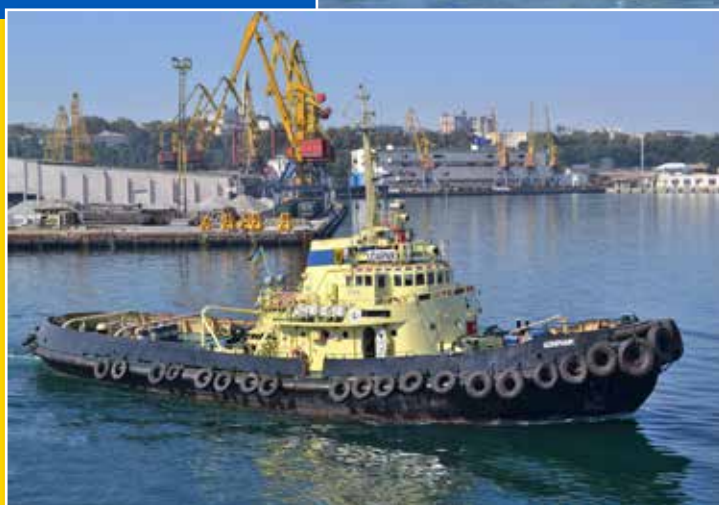
UDARNIK was a product of Brodogradiliste Tito. 35,43 / 30,00 x 9,21 x 4,50 m. Draught 3,17 m. 2x 7 cyl. B&W Alpha 7-26MTBF40, total output 2.316 bhp. 1992 to Odessa Commercial Sea Port
