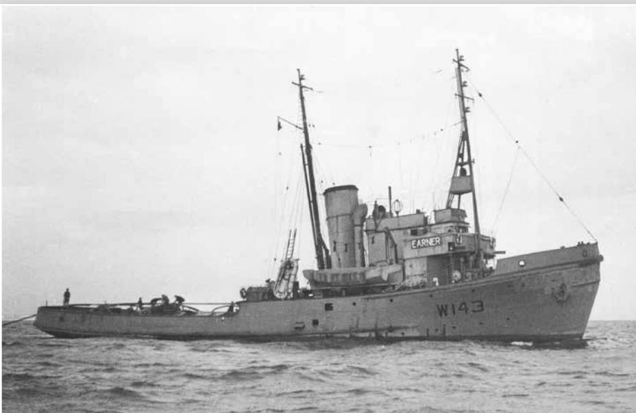
EARNER is an Assurance-class rescue tug built in 1943 by Cochrane. 700 t. displacement. 1.350 ihp triple-expansion. 13 knots. Armed with 1x 3" AA, 2x 20 mm AA and 2x 2 machine guns
