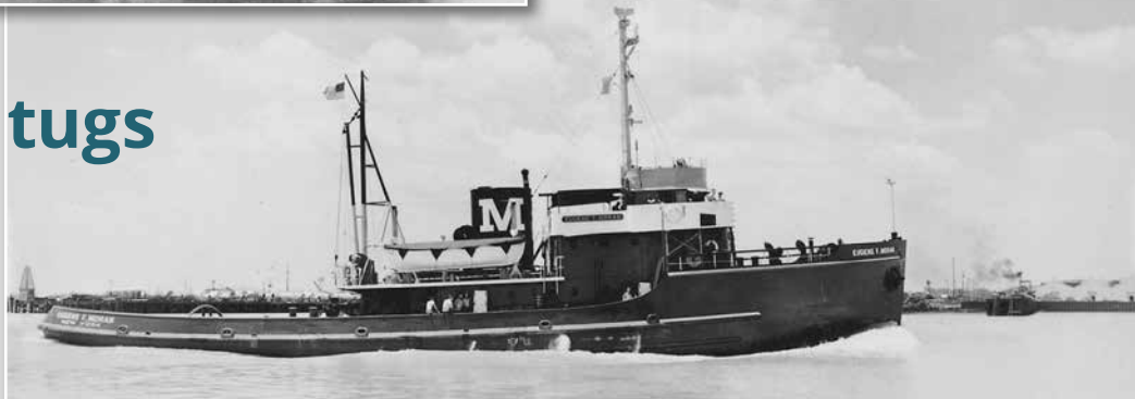
EUGENE F. MORAN is the former ATA type rescue tug FAVOURITE (W 119), one of the U.S. lend/lease tugs delivered to the U.K. 783 t. displacement. Built 1942 by Gulfport Boiler. Diesel-electric 1.875 bhp. 14 knots. Armed with 1x 3" AA, 2x 20 mm AA
