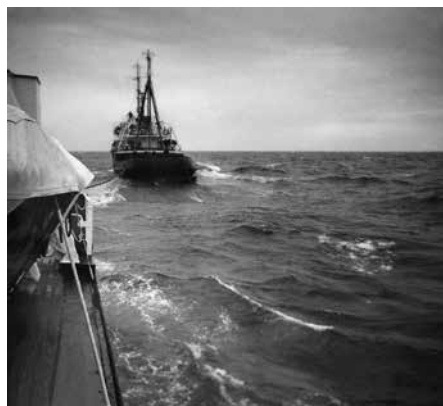
BARENTSZ-ZEE as seen from CLYDE. The towing connection visible to the right, to the left the fuel hose
