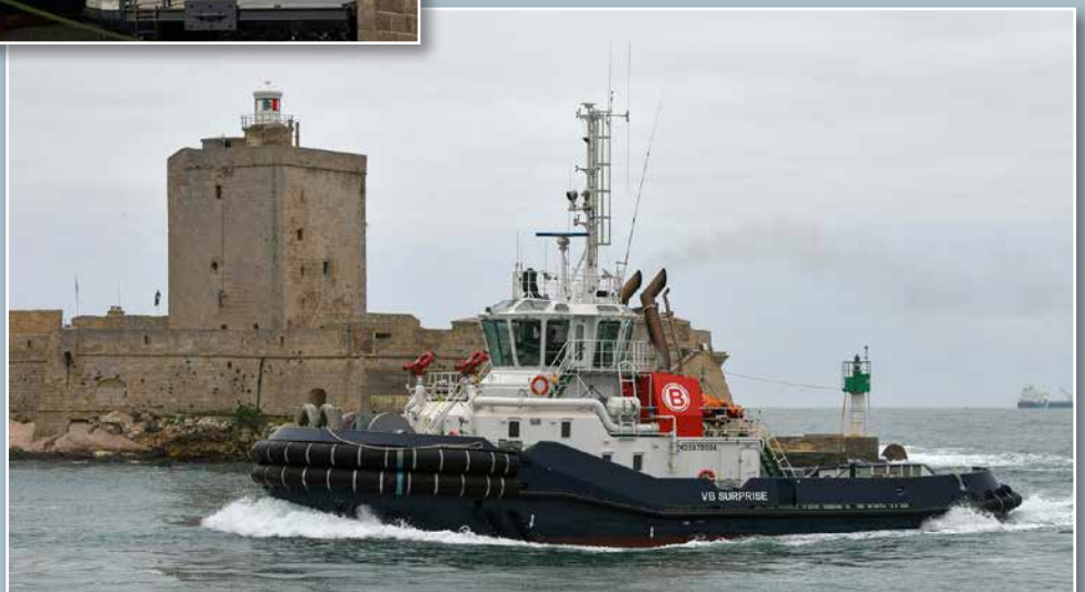
VB SURPRISE - seen here in February, 2021 - was completed in December, 2019, by Chantiers Piriou. The 30 x 10 m stern drive tug has a bollard pull of 73 tonnes. Her direct sister at Fos is VB ACHERON photo: via Wim Plokker
