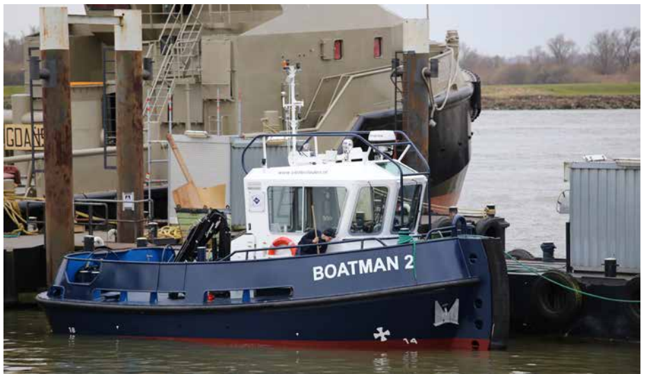
BOATMAN 2 was built by Damen Shipyards Changde as a stock vessel. The Corps van Vletterlieden (Boatmen Association) at Umuiden signed the contract on 2 October, 2020. The Stan Tug 1004 (bn 501113 - 4 ttp - 8 knots) was outfitted at Damen Hardinxveld to the owner's special requirements, including a crane, gen set and coupling winches. Seen here at Hardinxveld prior to delivery in 2021
