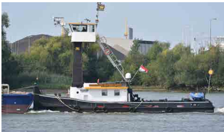
GEERTRUIDA VAN DER WEES on 1 August, 2024, with raised wheelhouse. Dimensions 21,46 (oa) x 6,97 (oa). Draught approx 2,20 m. Main engines 2x Caterpillar total 714 kW / 971 bhp. Twin screw in nozzles. Built 1979 by Deltawerf, Sliedrecht. Operated by Van der Wees Watertransporten BV, Dordrecht
