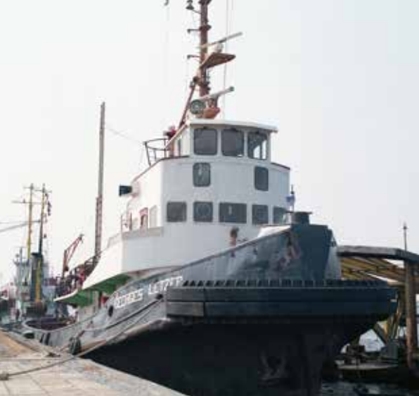
GEORGES LETZER after the 1981 upgrade with secondary top deck wheelhouse and modified bow for shiphandling purposes photo: Leen van der Meijden
