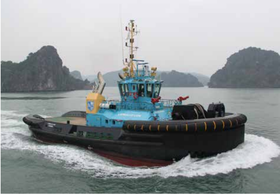
LAMNALCO LION – sold with the company to Boluda. Built 2011 - Damen ASD Tug 3213 – 75,4 tpb – Bergen diesels – Rolls-Royce azimuthing thrusters in the stern photo: courtesy Damen Shipyards
