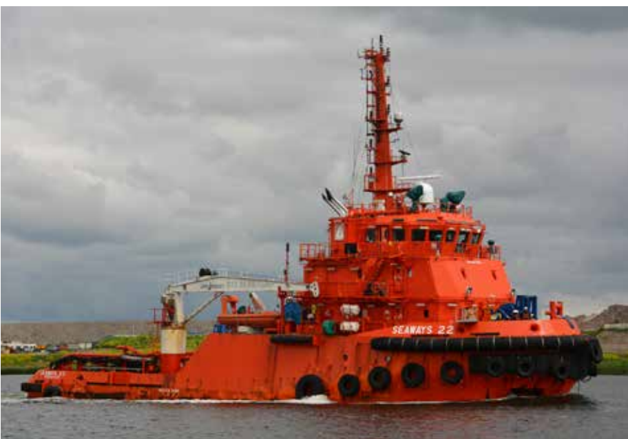
Seaways International's SEAWAYS 22 seen 13 June, 2018, en route Amsterdam. The 5.360 bhp - 81,75 tbp - 45,88 m oa - DP-1, OilRec-2, FIFI 1 is one of the vessels taken over by Kotug photo: Willem Koper
