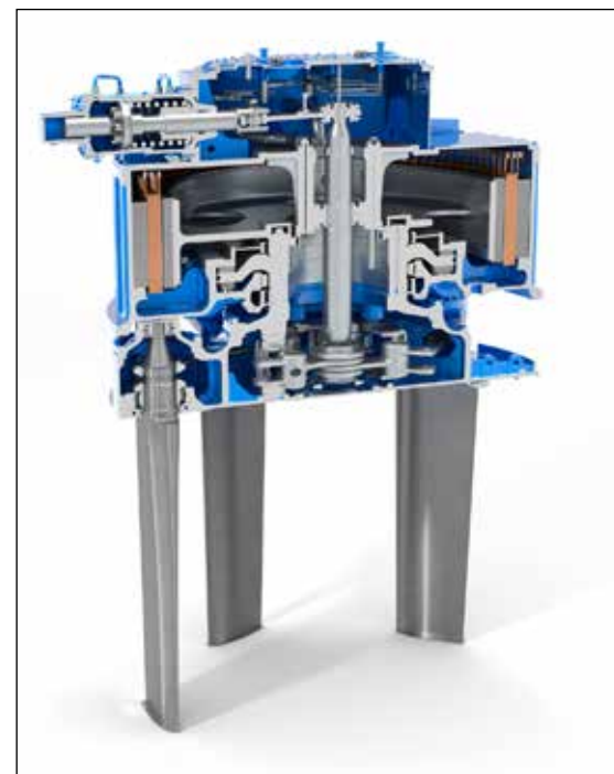
Sectional view of the newly-developed eVSP propulsion system artwork: courtesy Voith
