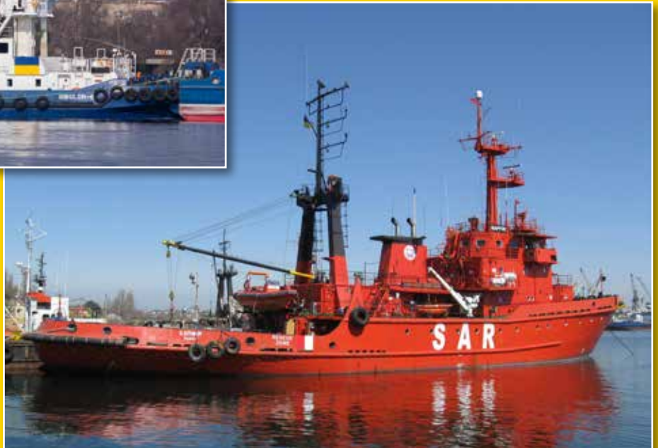
SAPFIR was built in 1988 by the Yaroslavl Yard. This is one of a series of 82 near identical vessels built at various yards for mainly state-owned companies and navies in the years 1970-1988. SAPFIR was completed in 1988 and one of six flying the Ukrainian flag. Currently owned by Marine Rescue Service and stationed in the Odessa region. 58,3 x 12,0 m - single f/p prop in nozzle - 2.920 bhp. The tug was reportedly seized by the Russian Navy on 25 February, 2022, when sent to Zmeinyi Island (known also as Snake Island) to search for survivors of the Russian shelling of the island. The Ukrainian garrison became famous when they over an open radio channel told the Russian commander to 'fu.. off' when ordered to surrender. While enroute the tug was diverted to assist a merchant ship being attacked by a Russian warship. Her present whereabouts are unknown.
