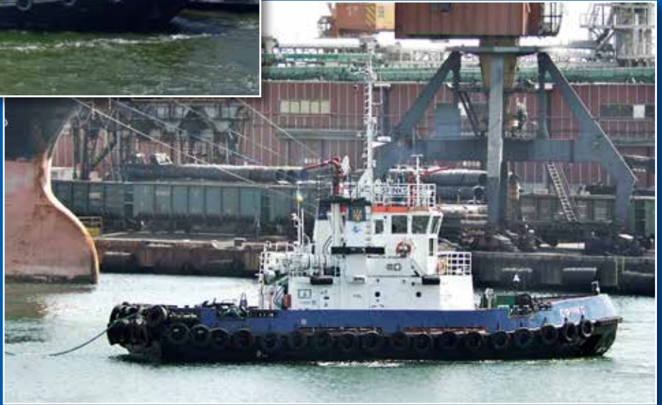
SFINKS was built in 1989 by the Apatin Shipyard (former Brodogradiliste 'Boris Kidric') in Serbia. 165 GT - 23,5 x 9,0 m - M.A.N. diesels. Output 816 bhp. Owner Black Sea Shipping. Ukraine flag.
