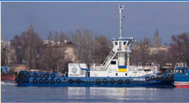
The NIBULON-6 pushboat was completed in 2014 by the Okean Shipyard for account of the Nibulon Agricultural LLC. 2x Mitsubishi diesel - output total 3.453 bhp - 37,2 x 11,2 m. Propulsion by two Berg azimuthing propellers - Ukraine flag.
