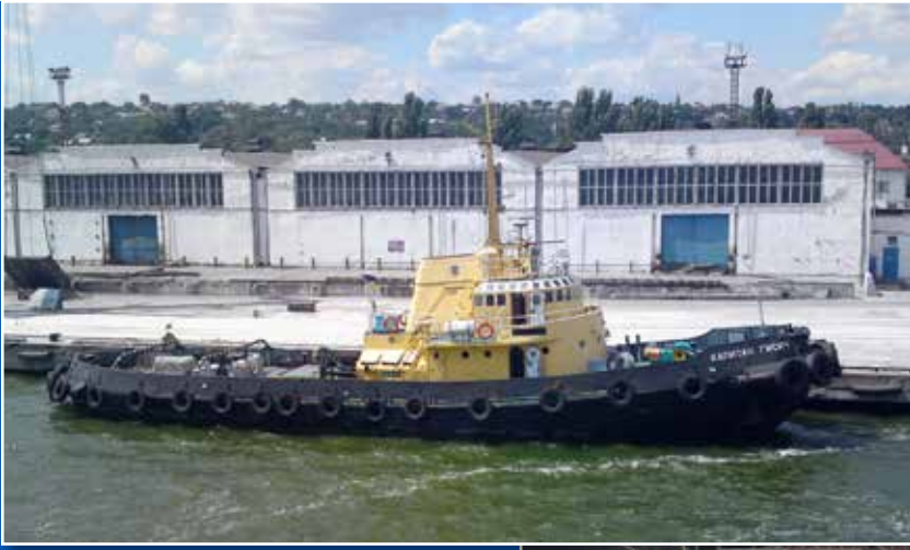
KAPITAN GISICH is another product of Brodogradiliste Tito. Built in 1970 the 35,4 x 9,3 m tug is fitted with 2x M.A.N. diesels. Output 2.316 bhp total. Twin screw. Owned by the Mariupol Commercial Sea Port.
