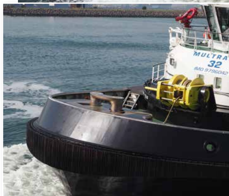
The travelling winch of MULTRATUG 32
