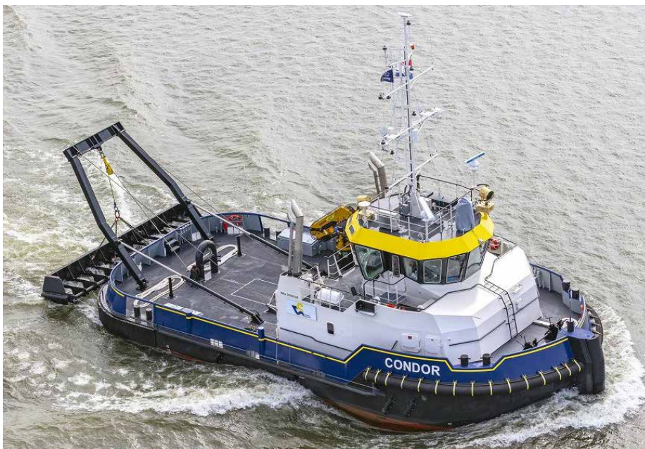
The Voith-driven EuroTractorTug CONDOR for Verbeke is a product of Neptune Marine, Aalst
