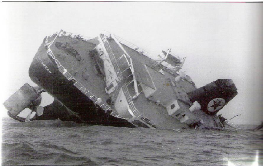
An enormous explosion occurred which blew the tanker in half, her bow section immediately and her stern section following about twelve hours later.
