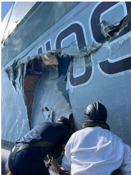
DAMAGE TO BANGOR'S HULL
