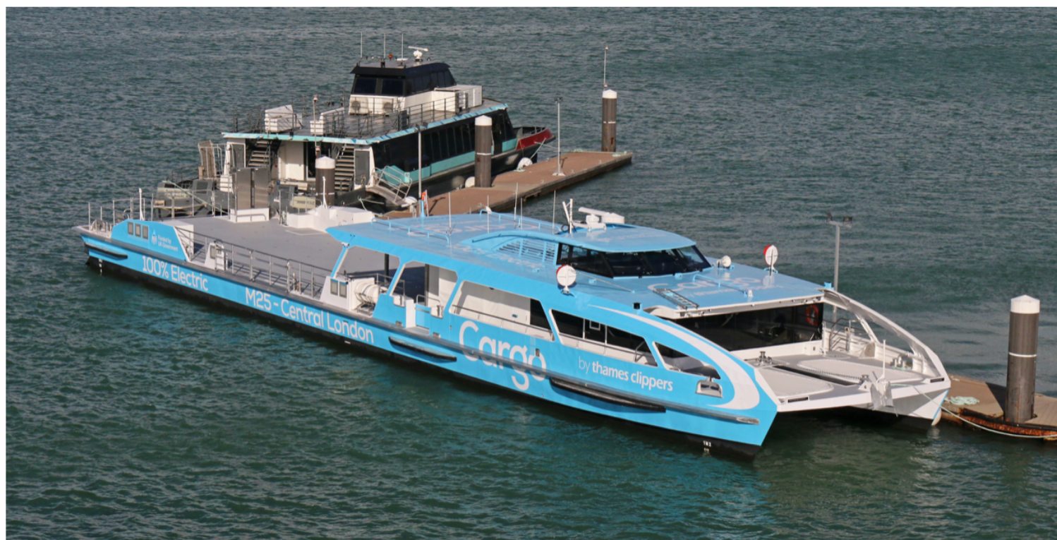
LIGHTNING CLIPPER - (no name on her, but she is showing on AIS). An electric cargo ferry for Thames Clippers for service on the Thames carrying light freight into the centre of London. Photo: Chris Brooks
