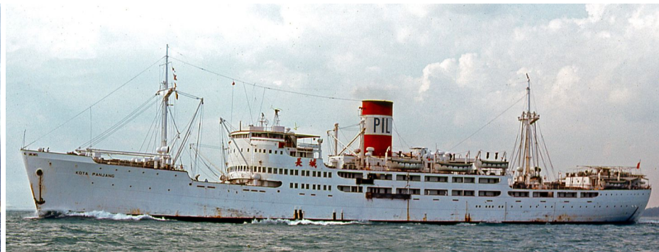
left: Kota Panjang's sister ship Kota Sahabat (ex-Taiyuan), anchored off Singapore with most of her lifeboats gone, and additional ventilators installed, including one up through the bridge, following conversion into a livestock carrier. (H. Stott Collection)
