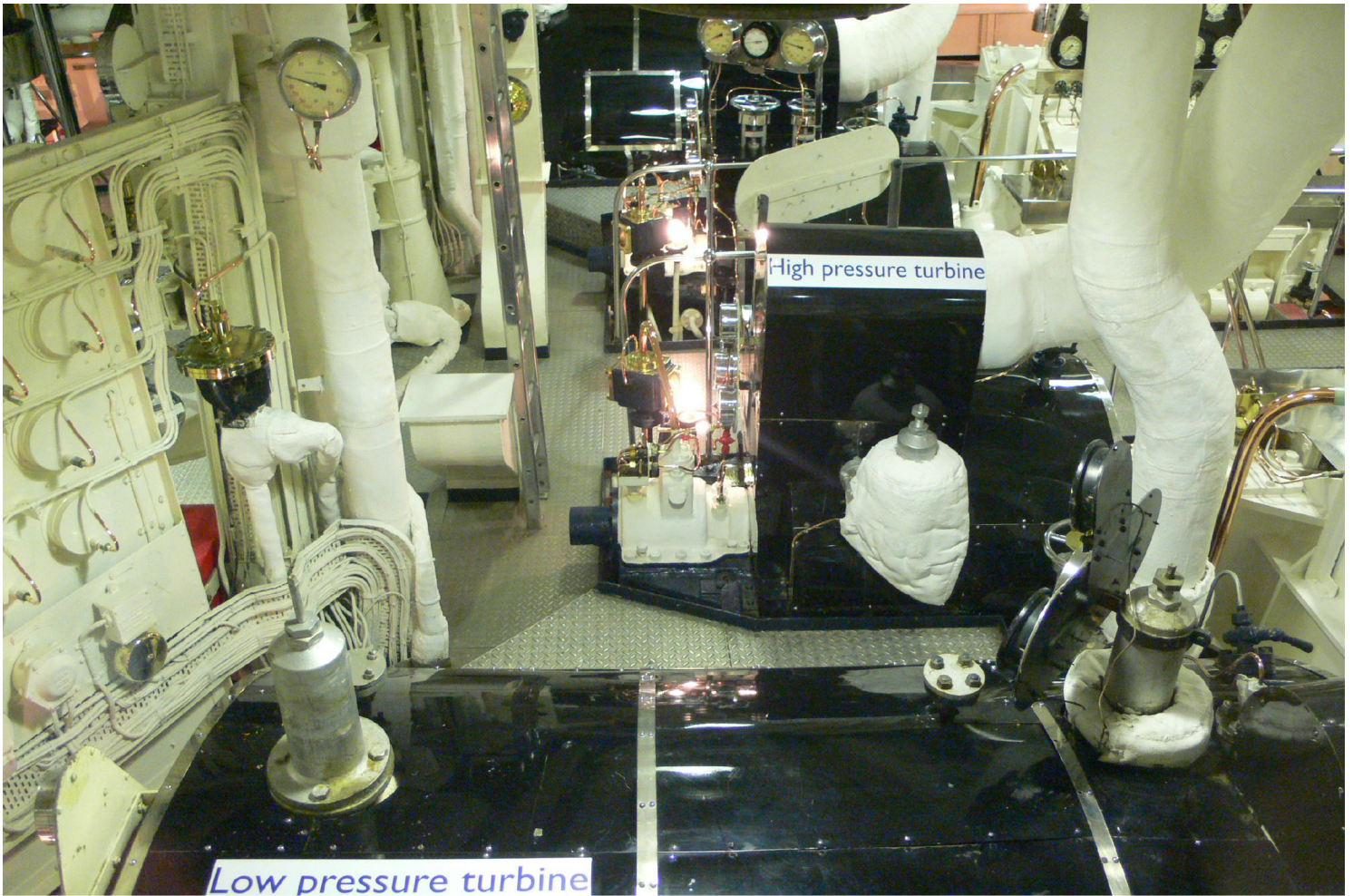
(above, and right) Two views of the engine room. Two Pametrada steam turbines, with 12,000 hp, were capable of driving the Britannia at a speed of up to 21.5 knots. Often times, the Queen would take guests here after dinner. (below) Should anything happen to the crew, or royal passengers, a fully-equipped operating theatre was onboard.
