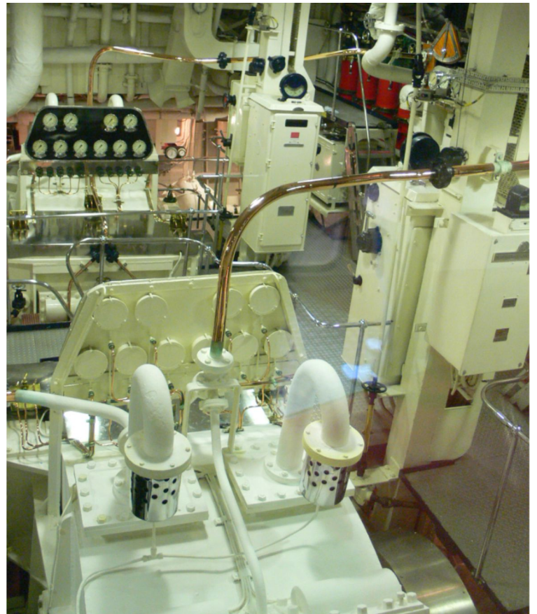
(above, and right) Two views of the engine room. Two Pametrada steam turbines, with 12,000 hp, were capable of driving the Britannia at a speed of up to 21.5 knots. Often times, the Queen would take guests here after dinner. (below) Should anything happen to the crew, or royal passengers, a fully-equipped operating theatre was onboard.
