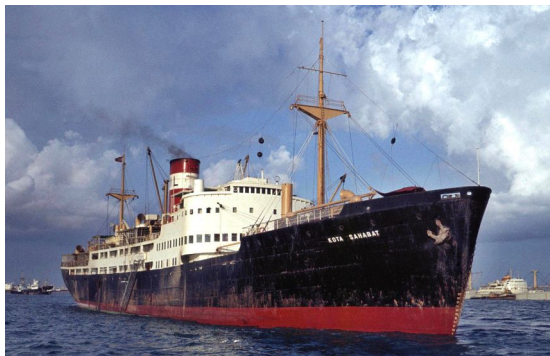
left: Kota Panjang's sister ship Kota Sahabat (ex-Taiyuan), anchored off Singapore with most of her lifeboats gone, and additional ventilators installed, including one up through the bridge, following conversion into a livestock carrier. (H. Stott Collection)
