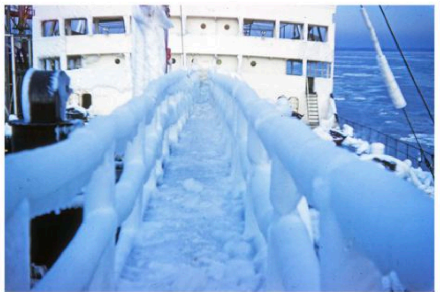
Iced-up catwalk ... Hours of chipping ice ahead
