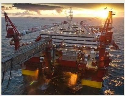
in May. Under the terms of this deal, **Floatel Superior** will be connected to the Balder FPU to be used as living quarters. The unit has been contracted for 13 weeks with a four-week extension option. The 2010-built **Floatel Superior** is a dynamically positioned (DP-3) semi-submersible accommodation and construction support vessel, which was constructed at the Keppel FELS yard in Singapore. Inge Bjørkevoll, VP Modifications Projects at Vår Energi, explained: "The 2021 campaign
