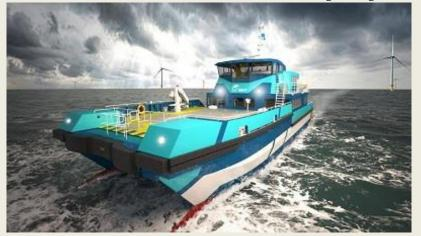
This will enable the vessel to play an increased role during the windfarm construction phases, with the ability to carry more equipment in support of the larger ships, BMT said. This design features BMT's Active Fender System, "an essential feature that enhances transfer capability in a wider range of sea states, as well as the safety of the technician transfer in
