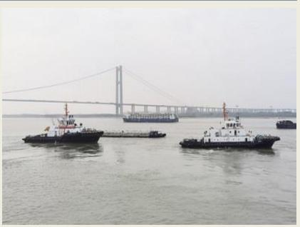
of 36.5m, breadth of 10.4m, depth of 4.6m, ahead pull of52t, astern pull of 48.2t, endurance of 1000nm and speed of 13.2kn. *(Source: Jiangsu Zhenjiang Shipyards)*
