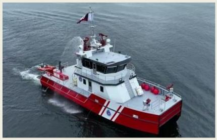
MetalCraft Marine of Ontario, Canada, has handed over a new aluminium catamaran firefighting and rescue boat to the Kuwait Fire Force. Designed by Walker Marine Design of the UK, Monjeb 2 has a length of 25.9 metres, a beam of 7.92 metres, and a draught of only 1.21 metres. The design is influenced by that of semidisplacement windfarm crewboats that operate in the
