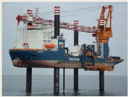
Van Oord's vessel Aeolus, responsible for drilling and pile installation pin operations for the jacket foundations on the Saint-Brieuc offshore wind farm, has completed its 2022 campaign. 40 positions of the Saint-Brieuc farm's jacket foundations that will support 62 Siemens Gamesa 8 MW wind turbines have been drilled and fitted with pin piles. After completing the operations, Aeolus returned to its home port in Vlissingen, the Netherlands,
