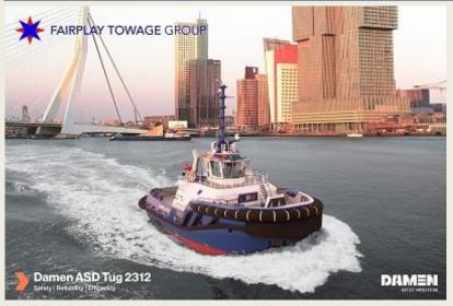
Fast delivery of harbour tug for operations in Port of Rotterdam. Engaging her impressive 70 ton bollard pull, Azimuthing Stern Drive tug Fairplay-93 will be performing towage services in Port of Rotterdam from the first months of 2023 onwards. Fairplay Towage has closed a lease contract with Damen Marine Services, who is able to deliver the vessel at very short notice following the contract signing on 27 October. The
