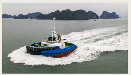
Portside Towing added a Bureau Veritas-classed azimuth stern drive (ASD) tug to its fleet in Jamaica during April 2022 towing, mooring, oil pollution control and firefighting. Damen Shipyards supplied Ajax, one of its ASD 2312 tugs, with an overall length of 22.8 m, beam of 12 m and draught of 5.6 m. Propulsion comes
