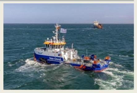
supplemented by innovative optimisations. The first of the two vessels will be commissioned in the first half of 2024. Energy management in this series of vessels was given special attention during the design phase. The water injection vessels will be equipped with a hybrid energy management system and will be able to store energy in batteries that can be used later for propulsion and other purposes.
