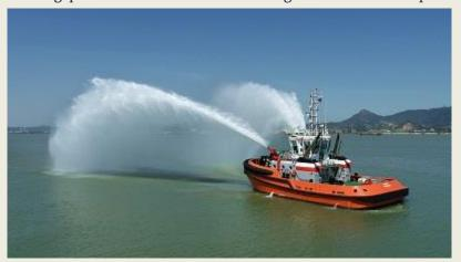
Peru. **Brujo** is a multipurpose, compact tug with 75 tonnes of bollard pull, FiFi1 fire-fighting system and two Kongsbergsupplied US255 P30 thrusters with fixed-pitch propellers. Also in Peru, PSA Marine is set to take delivery of PSA **Tallan**, a new RAmparts 2400W design tug with 70 tonnes of bollard pull, due to be delivered by the end of the year. In Brazil, Wilson Sons has
