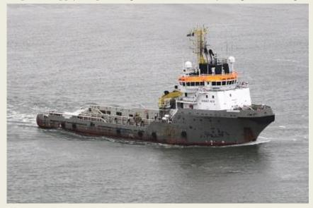
and renamed Sea Lynx. In sold Boskalis 2016 to Offshore Marine Services Papendrecht; BV. Netherlands and renamed Union Lynx. She has a length of 73.90 mtrs a beam of 16.40 mtrs and a depth of 8.00 mtrs. She has a total engine output of 11,038 kW (15,008 bhp) and performed a bollard pull of 177 tons. She is classed Det Norske Veritas. (Photo: Reinier van de Wetering)
