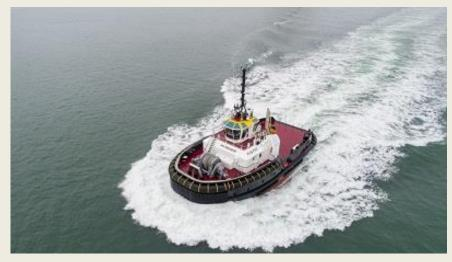
Plis Fos is an ASD 2813 tug IMO Tier IIIwith compliant propulsion and over 85 tons of bollard pull. Damen Shipyards delivered what it claimed is the most powerful tugboat of its type in the Caribbean, when it handed Plis Fos to its new owner in November 2022. This 388-gt escort tug is also one of the first in the region to comply with IMO Tier III
