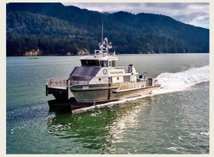
CDFW. The twin engine, fixed propeller patrol vessel will be built to Coast Guard standards. The hydrofoil assisted vessel from Teknicraft Design, Auckland. New Zealand, will combine innovative design features critical to modern maritime law enforcement and is based on the AAM-built Captain Murchison, built for the Texas Parks and Department. A Wildlife big feature included in the vessel is Teknicraft 's Rapid RHIB launching and retrieval system. This feature, integrated into the
