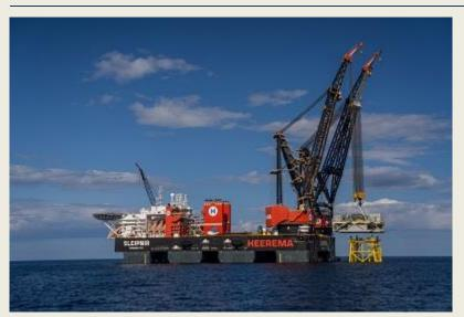
The world's largest semisubmersible crane vessel (SSCV), Heerema Marine Contractors' **Sleipnir**, is scheduled to place the offshore substation (OSS) topside on top of the jacket foundation that the vessel recently installed at the East Anglia Three offshore wind farm site in the UK. In August, Sleipnir completed the installation of the jacket foundation for the offshore substation and was expected to return to the UK project site in
