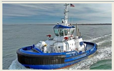
The Robert Allan Ltd (RAL)-designed Sirius is a cutting-edge escort tug for navigating crude tankers large through the Port Corpus Christi's channels. 31.48-metre-long, 31.86-metre-wide vessel features a triple-drive propulsion system with three engines, delivering 1,920 kW, and thrusters, achieving
