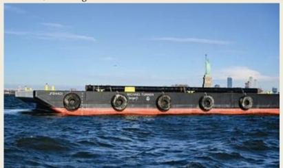
completely painted to prevent saltwater corrosion. On deck, the barge features a Manitowoc 4100 Series II crane. The crane on the barge is a Manitowoc 4100 Series II. There are three spud wells, each with 60-foot-tall and 30-inch-diameter spuds. Coating throughout is by Carboline. "The christening of the Michael Turner ensures that his legacy lives on in the work he loved and the company he helped to
