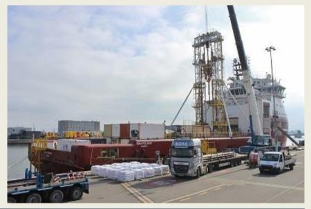
on the work deck. This rig is heave-compensated and can reach a drilling depth of 2,500 meters. The drilling rig stands above a 7.2 by 7.2-meter moonpool. Furthermore, the **Dina Polaris** is equipped with a Rolls-Royce Class 2 dynamic positioning system. The charter contract for the vessel was recently extended until 2030. (Source: www.maritiemdenhelder.eu; Paul Schaap)
