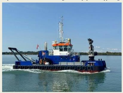
marine construction and offshore operations, including winches, an A-frame, a Heila deck crane and a plough. Willdiscover has two Volvo Penta D16 main engines compliant with IMO III regulations, developing 625 kW at 1,900 rpm, 1,650-mm diameter propellers in nozzles and an 80kW bow thruster. An anchor handling and towing winch, split-drum winch with a pull of 70 tonnes at the first layer, a tugger winch and a 25-tonne towing hook are fitted on
