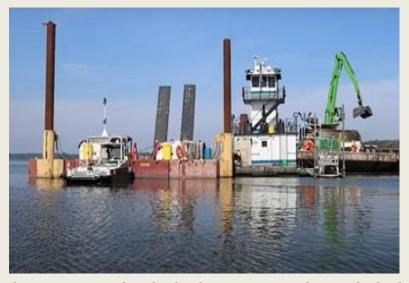
existing embankment from wind and wave erosion. The island is being constructed using dredged material from the 9-foot navigation channel. Work on the multi-million-dollar project in Pool 2 kicked off in early 2025 and is anticipated to be done by the fall of 2027. Watch the YouTube video HERE (Source: Dredging Today)
