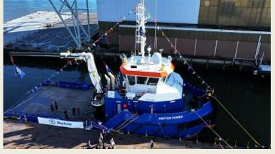
**Power**, following its construction by the Dutch designer and shipbuilder. This 34.2-m vessel was built to Neptune's EuroTug 3413 design with a bollard pull of 70 tons, a beam of 13.4 m and a shallow draught. It has DP1-class dynamic positioning and hybrid propulsion including three main
