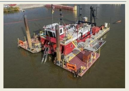
restore safe navigation by dredging the channels to their appropriate depths, between six and nine feet. The dredging, scheduled to begin in September, is expected to be completed in December 2025. Work will be conducted 24 hours a day, seven days a week. All material removed from the channels will be transported via pipeline and discharged into the Oyster Creek Confined Disposal Facility. (Source: Dredging Today)
