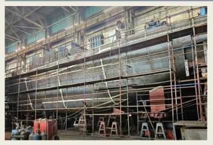
The third phase of construction of the Project 3262 icebreaking tug "Narvskaya Zastava" has been completed at the Nobel Brothers Shipyard in Rybinsk (part of the Kalashnikov Concern). reported to Sudostroenie.info on September 24, the concern's press service stated that the fully formed hull of the vessel was accepted by its customer—the Committee for Nature Management, Environmental Protection, and Ecological Safety
