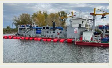
depths for vessel navigation along popular routes on inland waterways. The vessel was built at the Tsimlyansk Shipyard under a preferential leasing program. The Ts490DM1 design is equipped with a milling cutter and hydraulic ripper and is suitable for excavation at depths of 1 to 12 meters. (Source: Sudostroenie; Photo: Rosmorrechflot)
