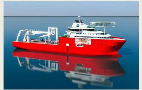
vessel, due for delivery at the end of 2027, is being billed the most powerful purpose-built TSV to date, with 24 MW of installed hybrid power and more than 180 tonnes bollard pull. newbuild is designed primarily for trenching operations in floating wind and subsea cable markets but will also be equipped for cable laying and repair work, the
