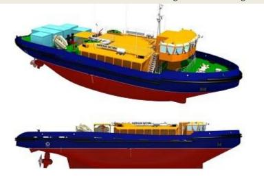
about 42.5 m; Length by design waterline (DWL) - 38.0 m; Width by DWL - 11.8 m; Height - 5.2 m; Draft by DWL - 3.8 m; Displacement - 655.7 t; Power plant - 2x1800 kW; Speed - about 11.0 knots; Crew - 8 persons; Endurance - 5 days. (Source: Sudostroenie; Photo: Kalashnikov Concern)
