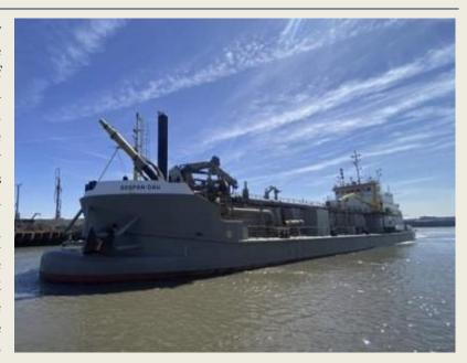
September to 3 October 2025. The survey vessel for these works is the 'ATHOS' (LOA 11.4m). The two vessels involved in the dredge works are the multi-cat 'WILLDISCOVER' (LOA 24.0m), carrying out the plough works, and the Trailer Suction Hopper Dredger (TSHD) 'SOSPAN DAU' (LOA 72.8m). (Source: Dredging Today)
