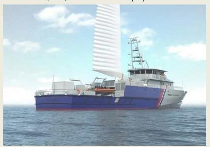
phase follows the tender win by **SOCARENAM-MAURIC** consortium in December 2024, and the official announcement in January 2025, with the task to deliver the next-generation OPV. MAURIC's team of naval architects and marine engineers completed the detailed arrangement study of the vessel, including an optimization loop for optimal sail positioning. This phase also enabled the finalization of active and passive stabilization systems
