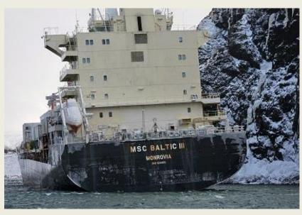
Containers with rotting food remain trapped on MSC Baltic III. Spoiled food in submerged containers aboard the MSC Baltic III is generating foul odours the grounded ship remains container stranded off Wild Cove. Newfoundland, more than seven months after it ran The 2,478-TEU aground. vessel has been sitting on the seabed since 15 February and cannot be refloated due to "significant" holes in its hull.
