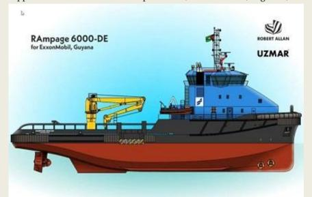
lifting at the deepwater floating production, storage, and offloading (FPSO) units located about 110 nautical miles off Guyana's coast. The vessels are being built by Uzmar in Turkey, with deliveries scheduled begin in early 2028. "Each vessel, of RAmpage 6000design bv architect Robert Allan, will be 60 meters long, with a ahead bollard pull exceeding 130 tons (astern
