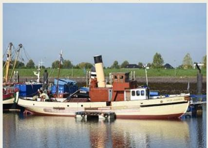
Wasserstraßenmachinenamt Rendsburg. (WMA) She mainly sailed on the Keizer Wilhelm Canal and Saatsee. The "von Bötticher" had a beautiful teak salon and deck. In the 1930s the ship was modernized and given a newly improved icebreaker bow. To this end, the hull was rebuilt partially reinforced with extra thick skin plates. In 1969 the ship was still in use at the WMA in Rendsburg, when it was purchased by the scrapyard
