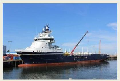
Once again, logistics service provider Peterson Den Helder has chartered a very large Norwegian supplier for a short period. This is the 96 meter long and 20 meter wide **Island Contender** from Island Offshore from Ulsteinvik. What is special about this ship is that it uses liquefied natural gas (LNG) as fuel for propulsion and can also sail on batteries. In 2012, the **Island** Contender launched at the Vard shipyard in Brevik, Norway. The working
