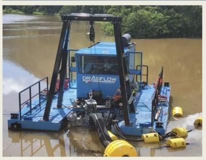
Italian Dragflow an of manufacturer dredging equipment - recently delivered and successfully commissioned a Drh85/180 cable dredge at a hydroelectric dam in Guinea. The Drh85/180, equipped with a dredging pump with a pumping capacity of up to 800 m3/h, will be essential for pumping mud and debris deposited on the bottom of the dam. The ambitious project provide clean aims accessible drinking water and a reliable source of electricity for the people Dabola and
