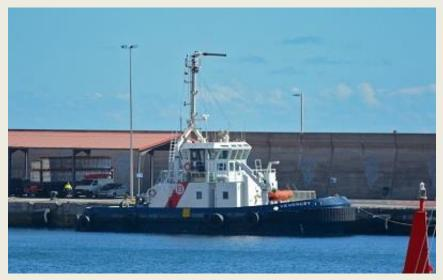
"Guerande", it comes from the Abeilles Nantes fleet and entered service in 1988. Of 198 gross tons, it measures 26.88 m in length, 9.12 m in width and 3.25 m in draft. She has a power of 3,220
