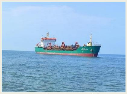
hoppers, bucket ladders and excavators. As reported, the company converted the TSHD into DredgePack for accurate dredge monitoring and DLM report. The installation, which was completed in 10 days, included replacing draft sensor in drydock as well as other sensors needed for the system
