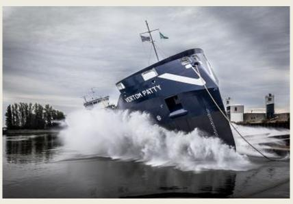
BN358 "Vertom Patty" was successfully launched Thecla Bodewes Shipyards on Friday 23 September. MV **Vertom Patty** is the first 7,000 DWT Diesel-Electric Multi Purpose Dry Cargo vessel of a series of six of the LABRAX design the Dutch yard is building. The vessel is ordered by Vertom, one of the leading short sea shipping operators within Europe. To emphasize the importance of this event, this first vessel in
