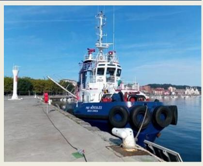
32 m in length, 11 m in width. and 5 m draft. She has Schottel diesel propulsion and maintains a speed of 12 knots.. (Source: Puente de Mando)
