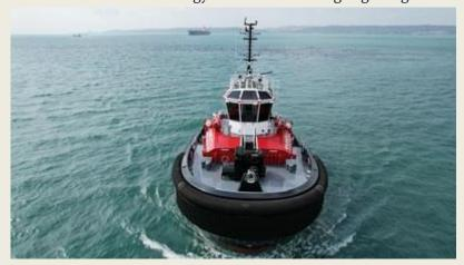
the type of deck equipment, including the winches and cranes owners require on vessels. Tugs with batteries and electric propulsion need additional power to drive electric winches and deck equipment. Owners are under pressure to cut their vessels' environmental footprint and minimise spills from the hydraulic oil used to control and power deck machinery. Tug operations have
