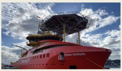
of 2023. The vessel is prepared for emission-free operations with a hydrogen-based propulsion system based on the liquid organic hydrogen carrier (LOHC) concept. The name "Nordri" comes from the Nordic mythology and represents one of the four characters (Nordri, Sudri, Vestri and Austri) holding up the sky after it was made by the Gods from the skull of Ymir. Edda Nordri will serve as mother vessel for wind turbine technicians as they perform commissioning and maintenance work on
