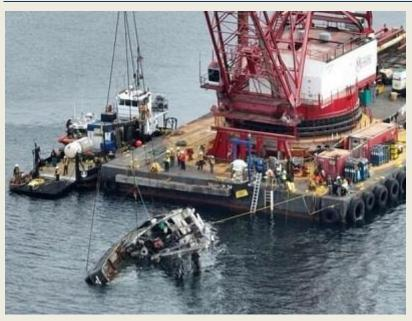
The salvage operation to remove the sunken fishing vessel **Aleutian Isle** from waters off San Juan Island have run into a snag. The salvage team placed lifting slings on the boat successfully hoisted it out of the water with a crane barge, but the operation has had to pause because the crew is having difficulty with dewatering. The **Aleutian Isle** was raised above the surface on Saturday afternoon, and salvage crews were able to pump out nearly 800 gallons of oily-water mixture. However,
