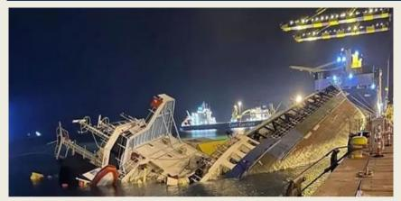
**SEA** General cargo ship **EAGLE** loaded with containers lost stability during offloading operation at Iskenderun Port, Turkey, either at night Sep 17, or early in the morning Sep 18. The ship, according to photos and video, rested starboard on pier, then listed and capsized portside, resting on bottom
