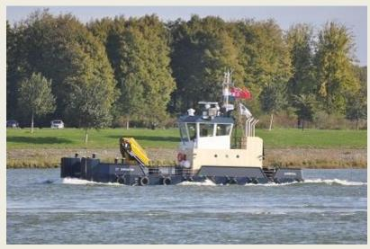
standardized design bollard pull with navigation notations Unrestricted navigation. The vessel has a length o.a. of 20.08 mtrs a length between pp of 18.55 mtrs a beam of 8.00 mtrs a depth of 2.75 mtrs and a dreaught of 1.86 mtrs. Her grt is estimated 70 tons and her dwt is 204 tons. The two Volvo Penta engines develops a total output of 882 kW (1,198 hp) and performed a free sailing speed of 8 knots. (*Photo: Ruud Zegwaard*)
