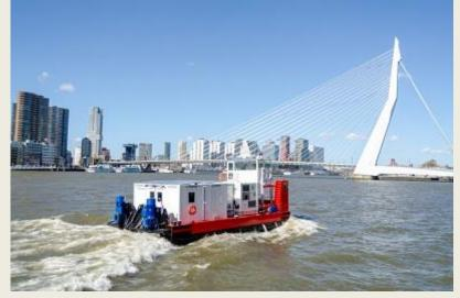
The **E-pusher** Type M is the first in a series of modular and scalable electrically powered pushboats, a very innovative concept which shows a different approach to sustainability in inland navigation. Padmos was commissioned to make the entire design of the first one and also build it. The design is highly modular, allowing parts to be produced completely in parallel and then assembled. The overall production process is thus
