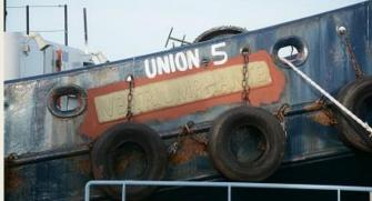
She has a length of 31.69 mtrs a beam of 10.04 mtrs and a depth of 4.76 mtrs. Her two ABC diesel engine produce a total output of 2,652 kW (3,606 bhp) and perform an free sailing speed of 12.6 knots and a bollard pull 47 tons ahead and 44 astern. She is a sister of the **Union 6** (Imo 9034987) built in 1993 on the same ship yard. *(Foto's: Richard Wisse)*
