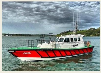
Safehaven Marine, an Irish builder of pilot, patrol and survey vessels, this week launched a new pilot boat for Svitzer's operations at Tanger Med 2 in Morocco. The newly built Svitzer Oued Laou is powered by a pair of 500horsepower Volvo Penta D13 engines. The 48-foot launch has an operational speed of 24.5 knots carrying seven pilots and crew. The vessel is self-righting and capable of operating in all weather conditions, the builder said. Safehaven Marine said the
