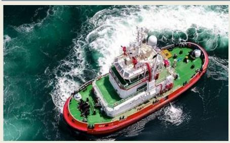
United Dubai, Arab **Emirates-headquartered** shipbuilder Grandweld Shipyard has delivered four harbour tugs to Specialities Construction (SCC) for operations in Shuwaikh Port in Kuwait. The four 27-m tractor tugs have Z-drive propulsion and 50 tonnes of bollard pull, an escortrated winch, deck crane and are equipped for oil
