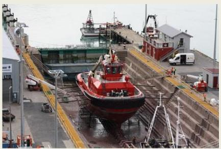
Wellington. The **Tiaki**, a Damen ASD 2411 design has a length of 24.55 mtrs a beam of 11.49 mtrs and a depth of 4.60 mtrs. The two Caterpillar 3516B-TA-HD main engines develops a total output of 4,200 kW (5,632 bhp) and performed a free sailing speed of 13.2 knots and a bollard pull of 68 tons. *(Photo: Alan Calvert)*
