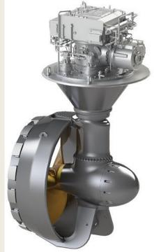
away the upper gearbox is reducing the mechanical losses and power consumption. Most of these vessels are diesel electric or fully electric, so it makes absolute sense to take away the upper gearbox," he said. The LE-Drive design offers more flexibility to the vessel designer. *(Source: Riviera by John Snyder)*
