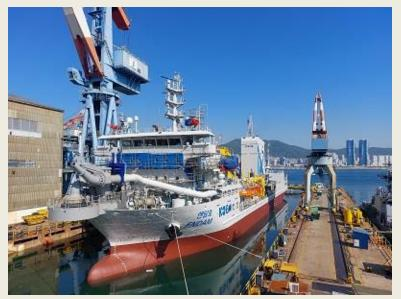
Damen Shipyards delivered a complete equipment package for the multipurpose vessel ENDAM. Owned by the Korean Marine Environment Management Corporation (KOEM), the newbuild combines emergency oil spill recovery activities with maintenance dredging tasks. With a 4,100 m3 hopper hold, the vessel was built by HJ Shipbuilding & Construction at its Busan yard and designed by KmsEmec. The mission equipment package provided by the Damen Technical Cooperation
