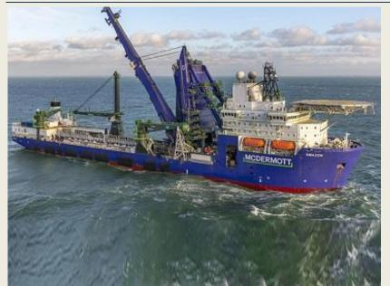
Royal IHC has completed a conversion that has transformed a 2014-built pipelay vessel into a J-lay vessel that owner McDermott International says will "redefine what's possible in deepwater construction." Now called the **Amazon**, the then **Ceona Amazon**, delivered by shipbuilder Lloyd Werft, Bremerhaven in 2014, was acquired by McDermott in early 2017 after it had been in layup since former owner Ceona went into administration in 2015. September the In
